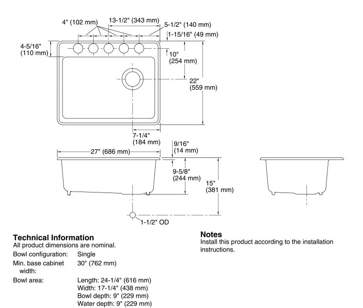
Number of deck<br/>holes:5Drain hole:3-7/8" (98 mm)Template:1244382-7, required, included
