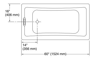
No change in measurements if connected with drain illustrated. (K-23856-NA)
