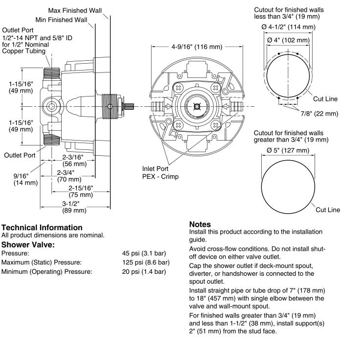
For finished walls greater than 1-1/2" (38 mm), install support(s) 3" (76 mm) from the face of the finished wall.
