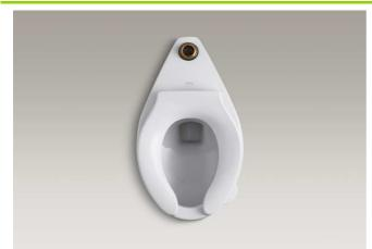
The elongated toilet bowl shall be made of vitreous china. Bowl shall be 28-1/4" (718 mm) in length, 14-7/8" (378 mm) in width, and 17-1/8" (435 mm) in height. Bowl shall be 10" (254 mm) or 12" (305 mm) rough-in with 1-1/2" top spud. Bowl shall feature 1.28 gpf (4.8 lpf) or 1.6 gpf (6.0 lpf) depending on flushometer specified. Bowl shall have 11" (279 mm) by 9" (229 mm) water area and 2-1/4" (57 mm) passageway. Bowl shall have optional bedpan lugs (-1).
