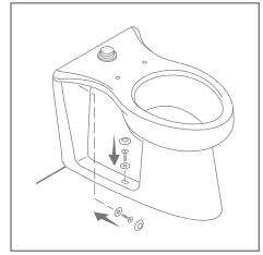
STEP 3 Place bowl onto bracket and connector system and secure in place.
