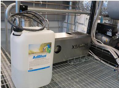
*A carefully collaborated dose of AdBlue breaks down nitrogen oxides into harmless water vapour and nitrogen.*
