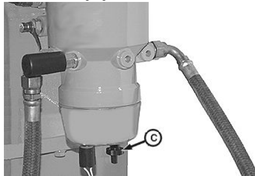
Draining Fuel Sediment Bowl (Earlier Engines shown)
