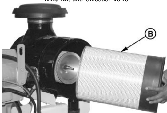
Replacing Primary Air Filter Element
