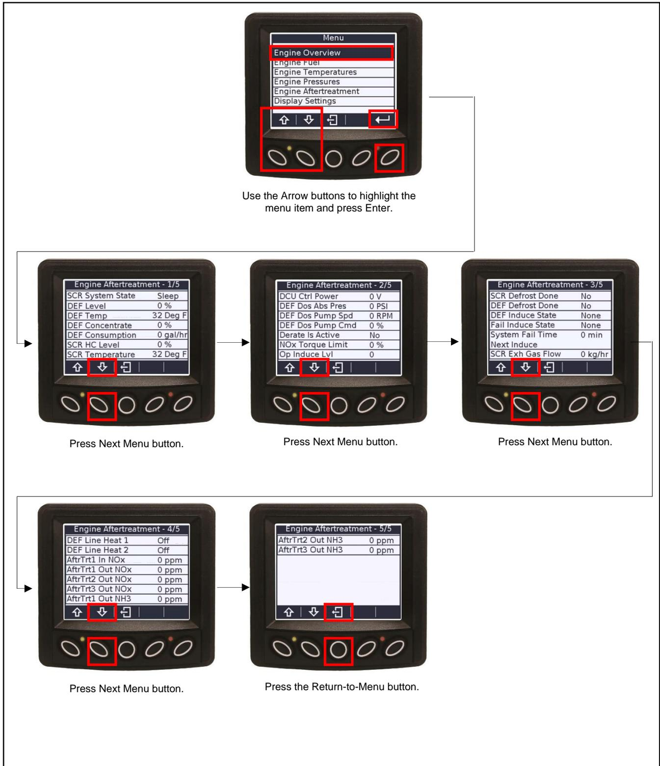
Figure 93 Engine Aftertreatment Navigation
