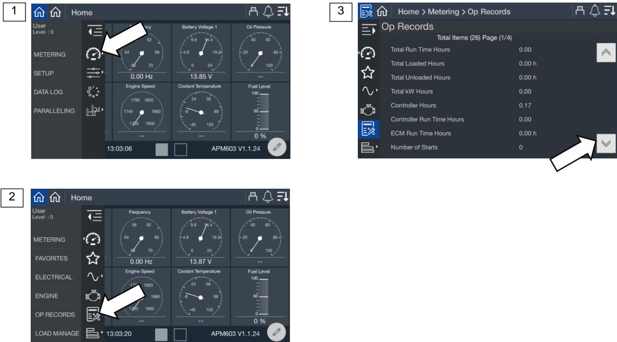
Figure 42 Metering Screen, Operation (Op) Records
