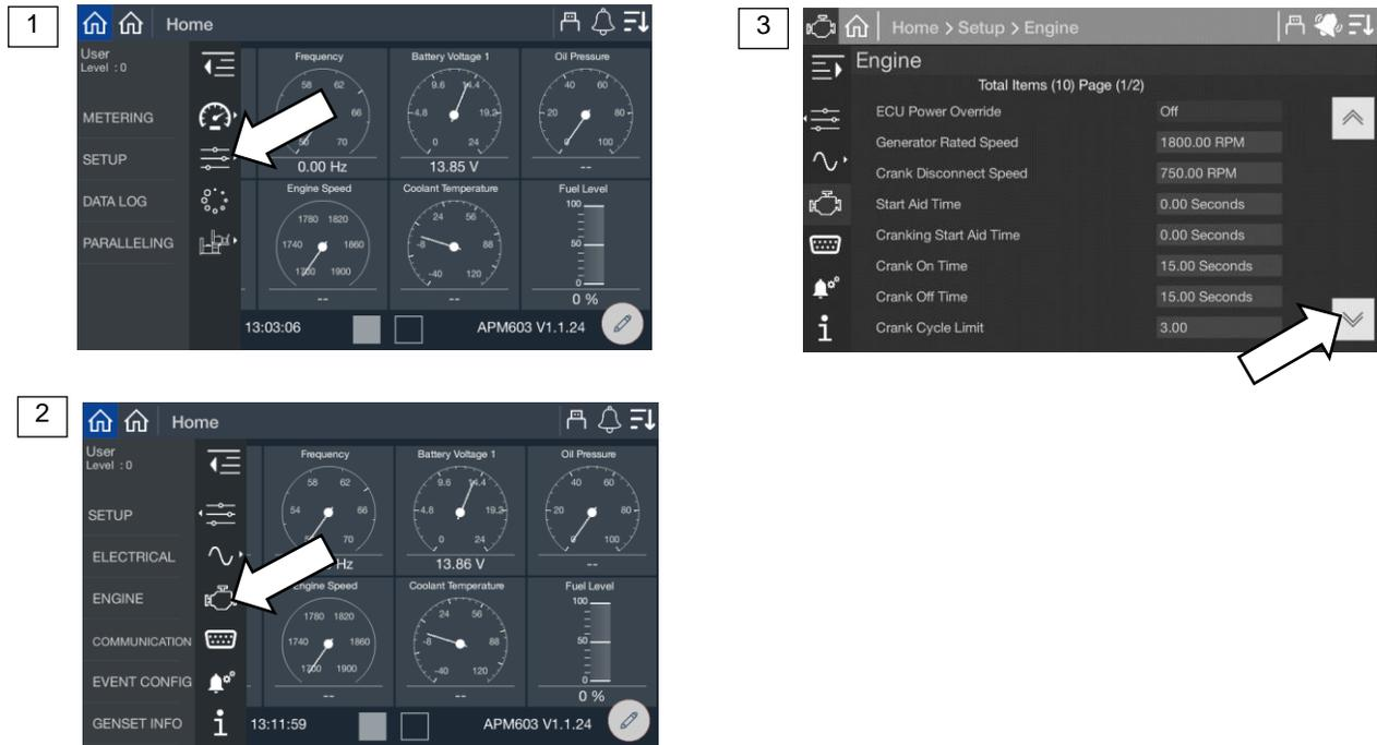
Figure 55 Setup Screen, Engine
