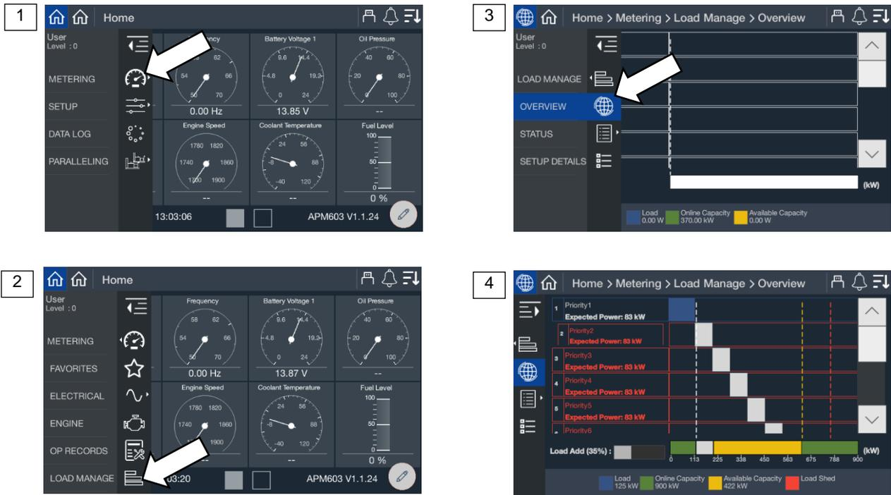
Figure 44 Metering Screens, Load Management Overview
