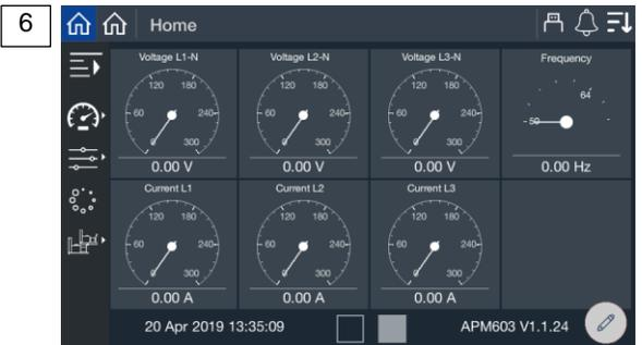
Figure 21 Adding Gauges to the Home Screen
