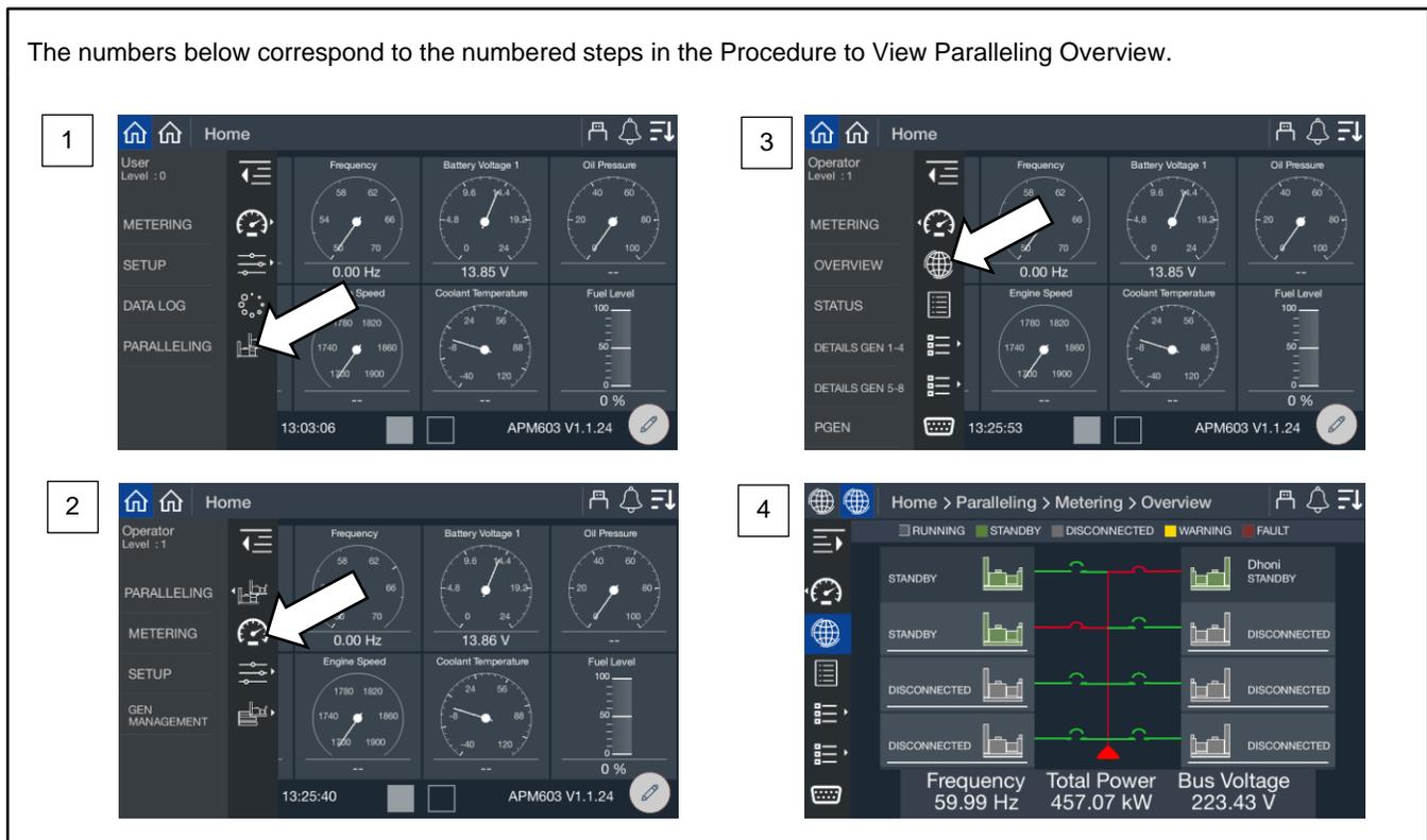
Figure 64 Paralleling, Metering, Overview Screen
