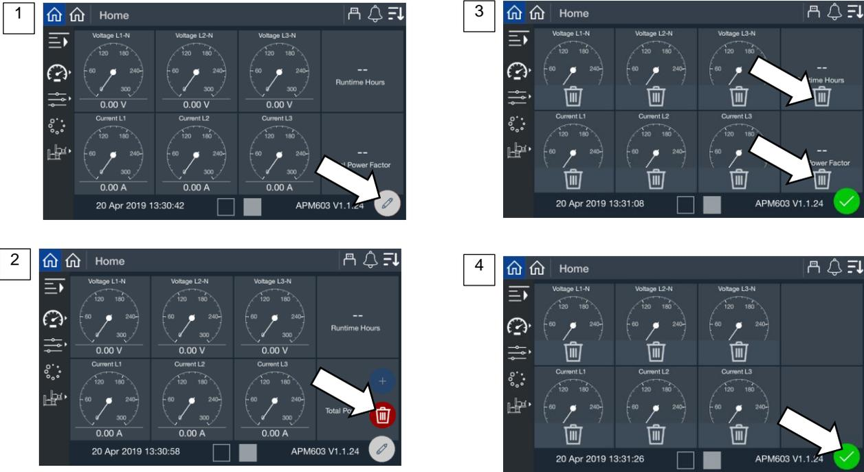
Figure 20 Removing Gauges from the Home Screen
