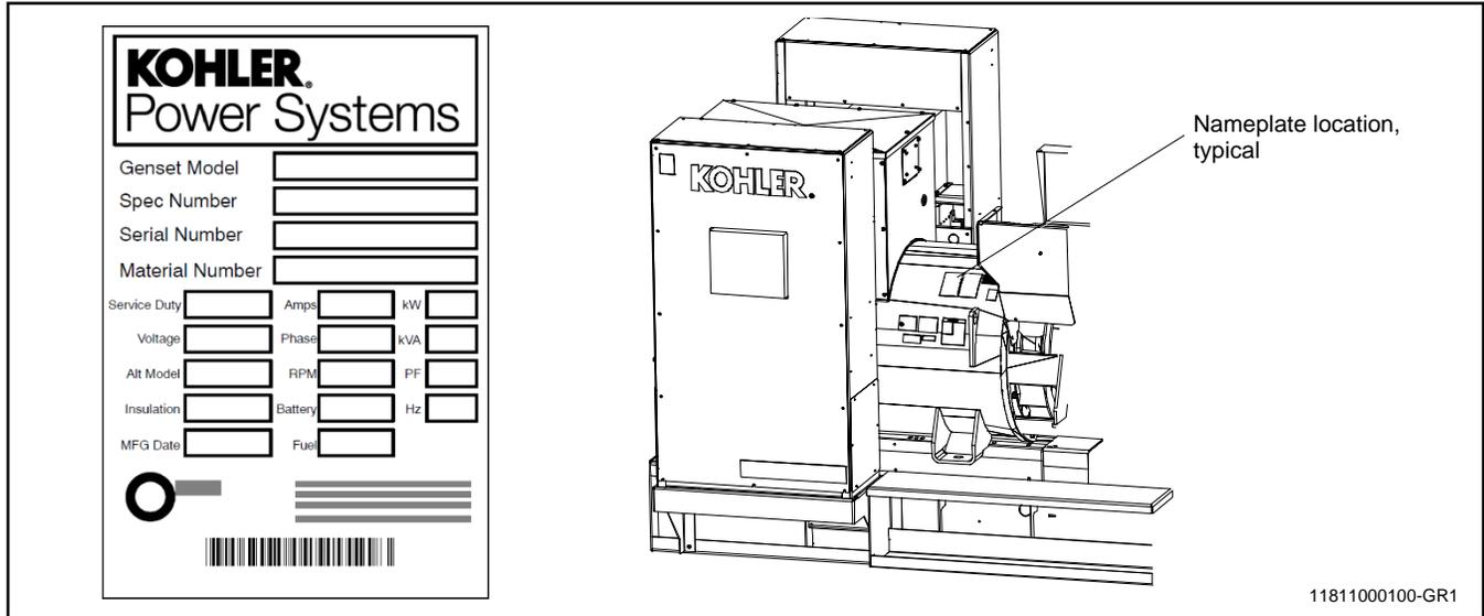
Figure 2 Generator Set Nameplate and Location, Typical
