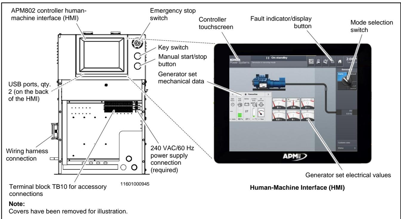
Figure 3 APM802 Controller and Customer Connection Box
