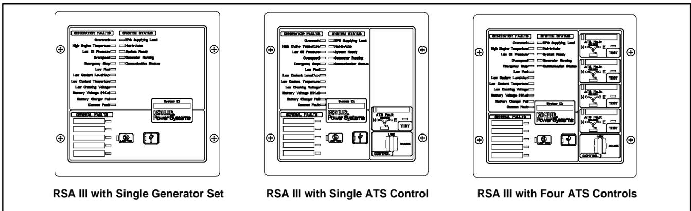
Figure 104 Remote Serial Annunciator (RSA III)
