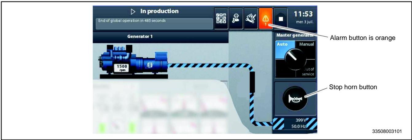
Figure 38 Appearance of an Alarm (warning)
