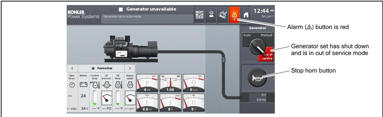
Figure 39 Appearance of a Fault (shutdown)
