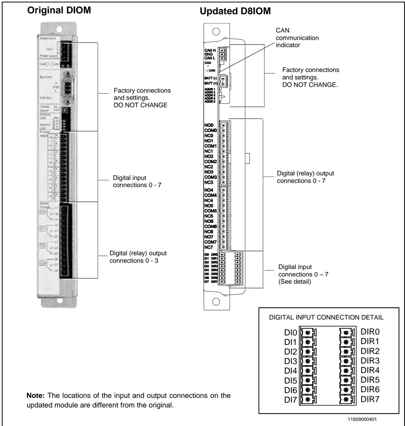
Figure 95 Digital Input/Output Modules, Original and Updated
