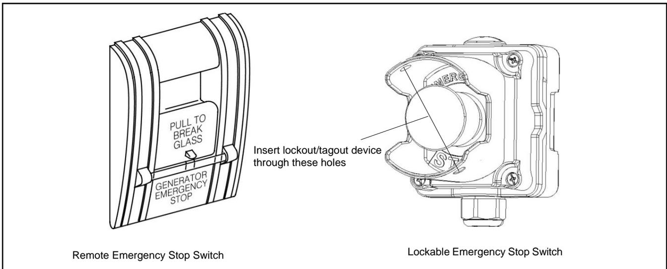
Figure 103 Remote Emergency Stop Switches
