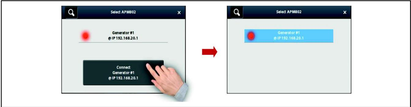
Figure 57 Selecting a Module from a Remote HMI
