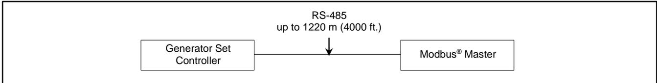
Figure 5 Modbus® Connections
