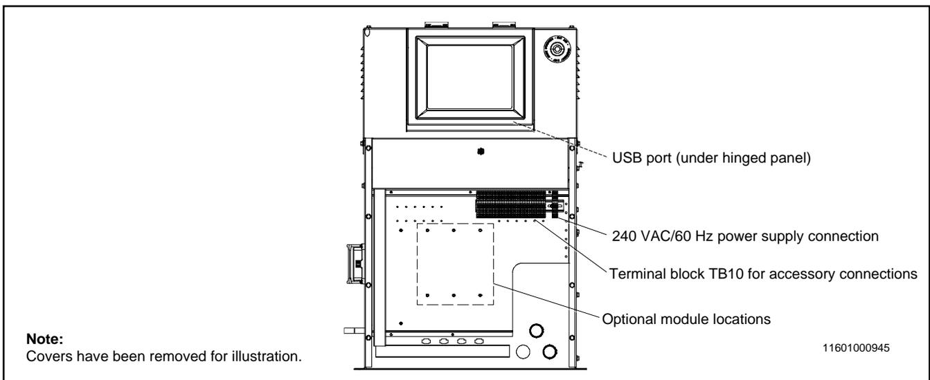
Figure 90 APM802 Controller and Customer Connection Box
