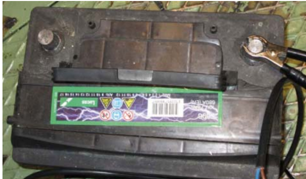
Image 2 – Earth clamp on battery negative terminal
