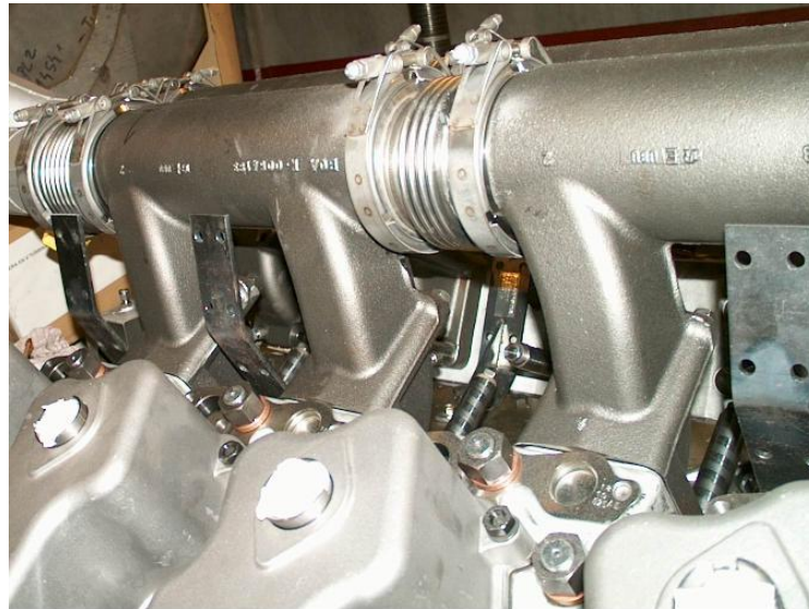
Fig. 1 Example of dry exhaust manifold on a V-engine
