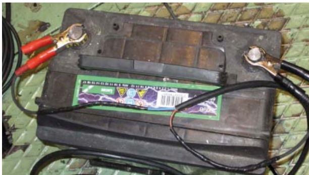
Image 3 – Red clamp on positive terminal of the battery
