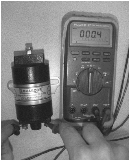
Fig. 1 - Measuring the resistance of the primary winding of an ignition coil ref. 76.64.302
