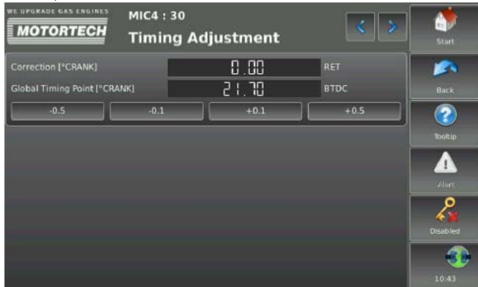
Fig. 14 – Adjusting the ignition timing
