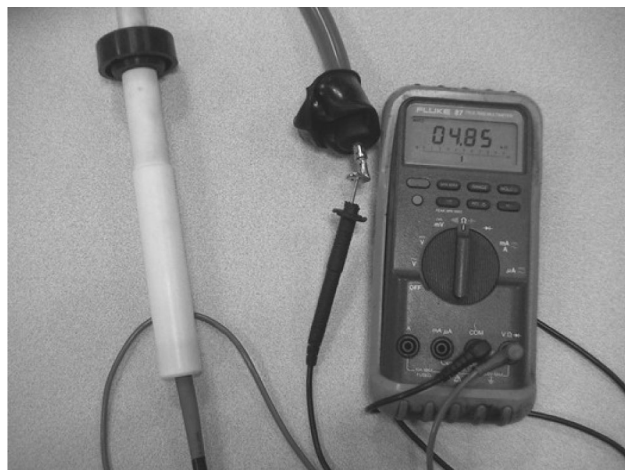
Fig. 3 - Measuring the resistance of a spark plug wire ref. 76.64.303
