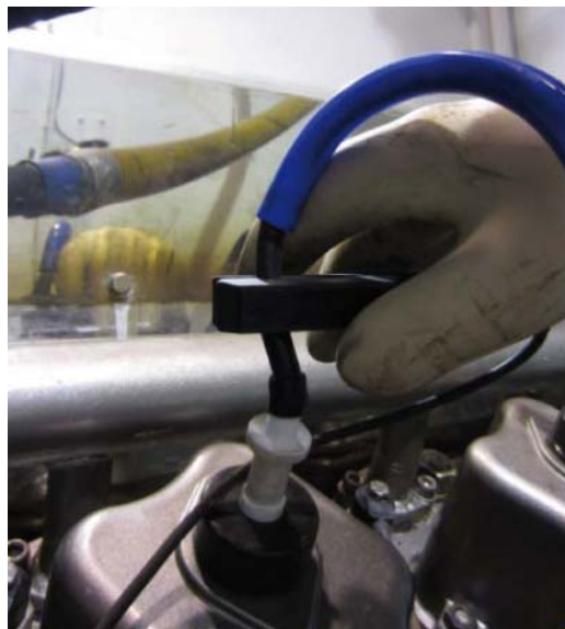
Image 5 – Connecting the clamp wearing high voltage gloves
