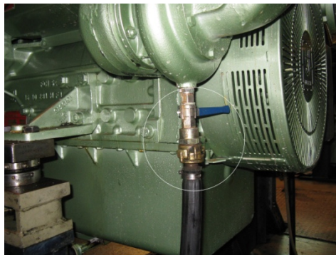
Fig. 5 - Typical hose/circuit connection for filling and draining the cooling system
