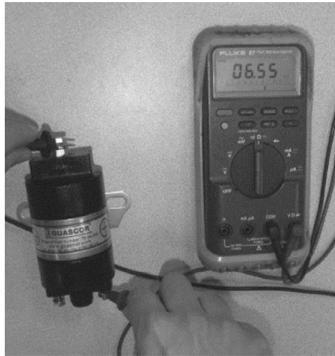
Fig. 2 - Measuring the resistance of the secondary winding of an ignition coil ref. 76.64.302
