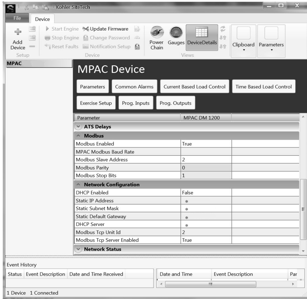
Figure 62 Communications Setup using Kohler® SiteTech™ Software (typical screen shown)
