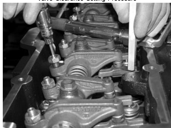
Checking Valve Clearance Using Bent Feeler Gauge
