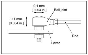
Fig. 8-12 Ball Joints For Looseness - Inspect
