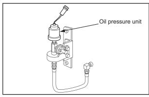
Fig. 2-6 Oil Pressure Unit
