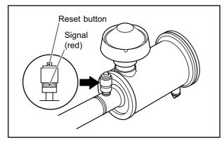
Fig. 8-30 Air Cleaner - Check for Clogging
