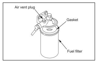
Fig. 8-10 Fuel Filter - Replace
