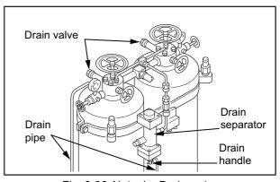
Fig. 8-36 Air tank - Drain water
