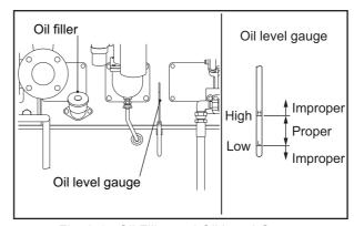
Fig. 3-15 Oil Filler and Oil Level Gauge
