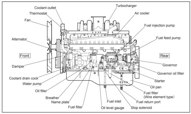
Fig. 2-1 Engine Left Side View
