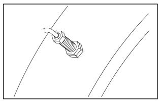
Fig. 2-12 Revolution Detection Pickup
