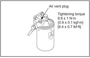
Fig. 3-3 Fuel Filter - Bleed Air
