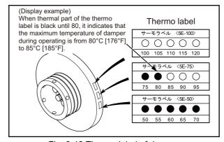
Fig. 3-19 Thermo label of damper
