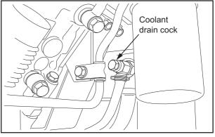
Fig. 3-10 Coolant Drain Cock (Engine)
