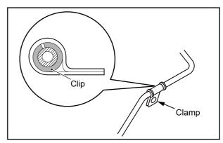
Fig. 8-20 Oil Pipe and Clip - Inspect and Replace
