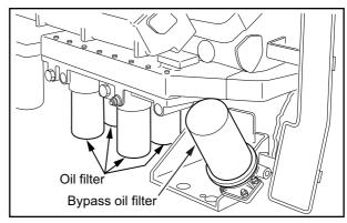
Fig. 8-17 Oil Filter and Bypass Oil Filter - Replace
