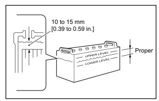
Fig. 8-31 Battery Electrolyte Level - Inspect
