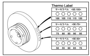
Fig. 8-3 Damper Temperature Management
