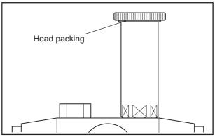
Fig. 3-6 Priming Pump Head Packing
