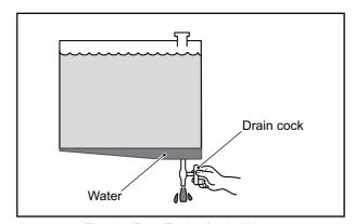
Fig. 8-4 Fuel Tank - Drain Water
