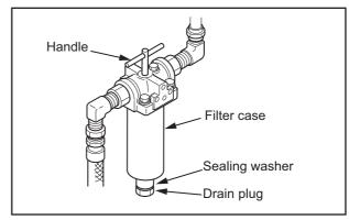
Fig. 8-8 Fuel Filters (Wire-element Type)
