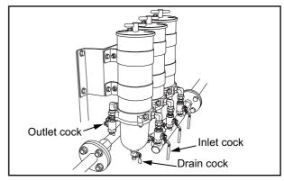
Fig. 8-5 Water Separator - Drain Water
