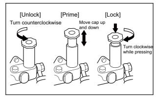
Fig. 3-1 Priming Pump - Handle
