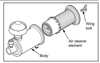
Fig. 8-28 Air Cleaner Element - Remove
