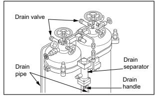
Fig. 3-17 Air Tank - Drain Water
