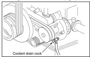
Fig. 3-11 Coolant Drain Cock (Water Pump)
