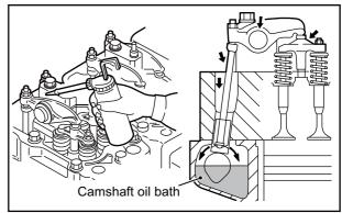
Fig. 3-8 Pouring Engine Oil on Valve Mechanisms and Chamber
