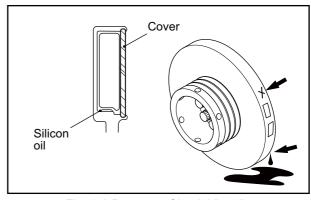
Fig. 8-2 Damper - Check Visually
