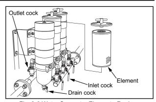
Fig. 8-6 Water Separator Element - Replace
