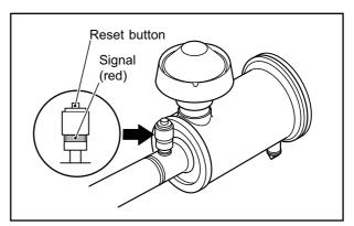
Fig. 3-16 Air Cleaner - Check for Clogging
