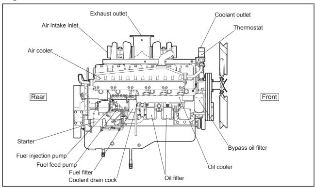
Fig. 2-2 Engine Right Side View
