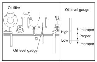
Fig. 8-16 Oil Filler and Oil Level Gauge
