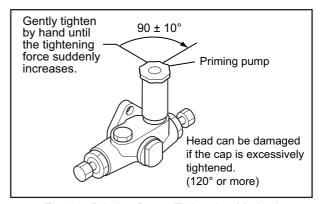
Fig. 3-5 Priming Pump Tightening Method
