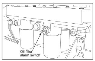
Fig. 2-11 Oil Filter Alarm Switch
