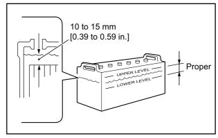
Fig. 3-12 Battery Electrolyte Level - Inspect
