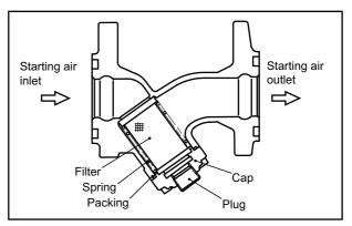
Fig. 8-35 Air Strainer - Drain Water and Clean
