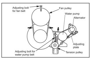
Fig. 8-1 Adjusting the Belt Tension
