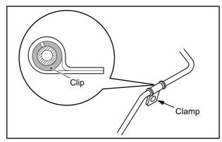
Fig. 8-15 Low Pressure Fuel Pipe and Clip - Inspect
