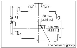
Fig. 10-2 Engine's center of gravity (standard specification)
