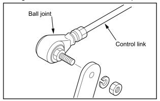
Fig. 8-13 Fuel Control Link - Remove
