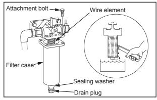
Fig. 8-9 Inside of Fuel Filters (Wire-element Type) - Clean
