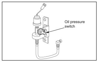
Fig. 2-9 Oil Pressure Switch
