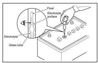
Fig. 8-32 Specific Gravity of Battery Electrolyte - Check
