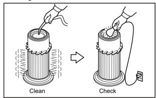
Fig. 8-29 Air Cleaner Element - Clean and Check
