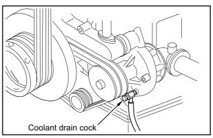
Fig. 8-23 Coolant Drain Cock (Water Pump)
