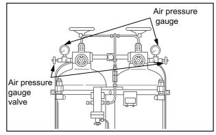
Fig. 3-18 Starting Air Tank Air Pressure - Check
