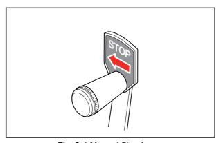
Fig. 2-4 Manual Stop Lever
