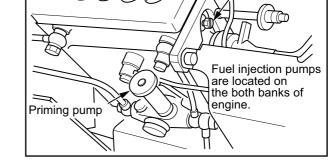
Fig. 3-4 Fuel Injection Pump - Bleed Air
