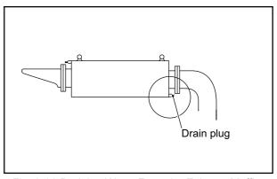
Fig. 8-26 Draining Water From the Exhaust Muffler
