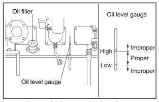
Fig. 3-7 Oil Filler and Oil Level Gauge
