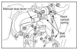
Fig. 3-14 Fuel Control Link - Check
