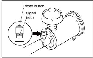
Fig. 8-27 Air Cleaner - Check for Clogging
