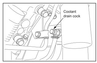
Fig. 8-22 Coolant Drain Cock (Engine)
