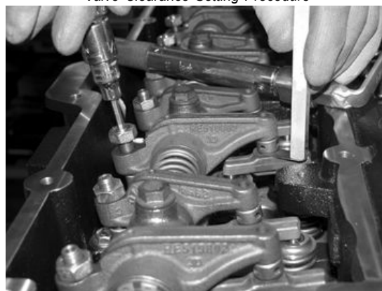
Checking Valve Clearance Using Bent Feeler Gauge
