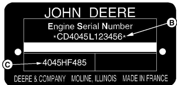
Saran Factory Engine Serial Number Plate
