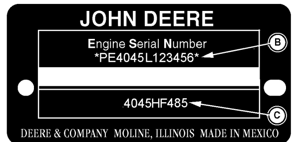
Torreon Factory Engine Serial Number Plate
