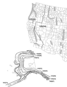
Figure 2.1 IBC Basic Wind Speeds: Basic Wind Speeds: Risk Category III and IV. Source: ASCE 7-10
