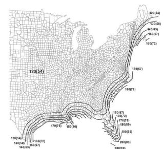
Figure 2.2 IBC Basic Wind Speeds: Basic Wind Speeds: Risk Category III and IV. Source: ASCE 7-10
