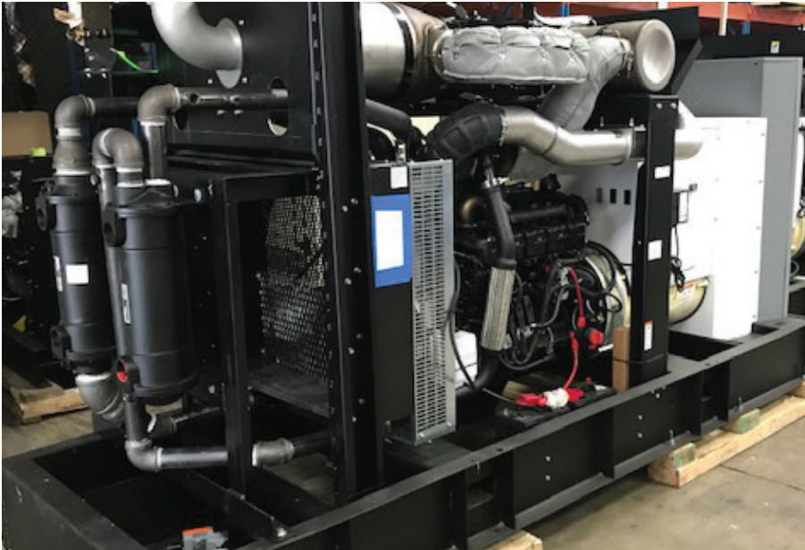
The heat-exchanger cooling system on the KOHLER 150 kW generator
