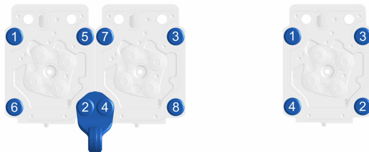
Fig. 101: Cylinder head tightening sequence
