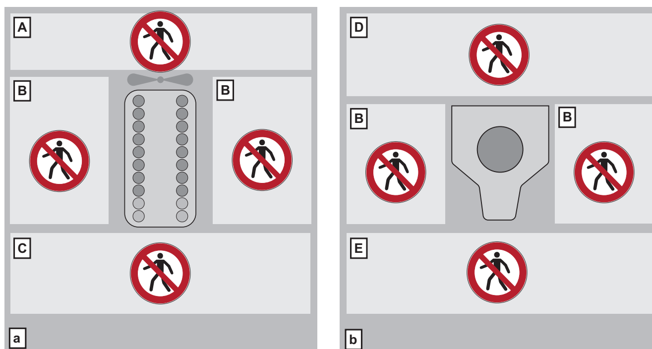
Fig. 1 Safety zones for the engine that is ready for operation or in operation
