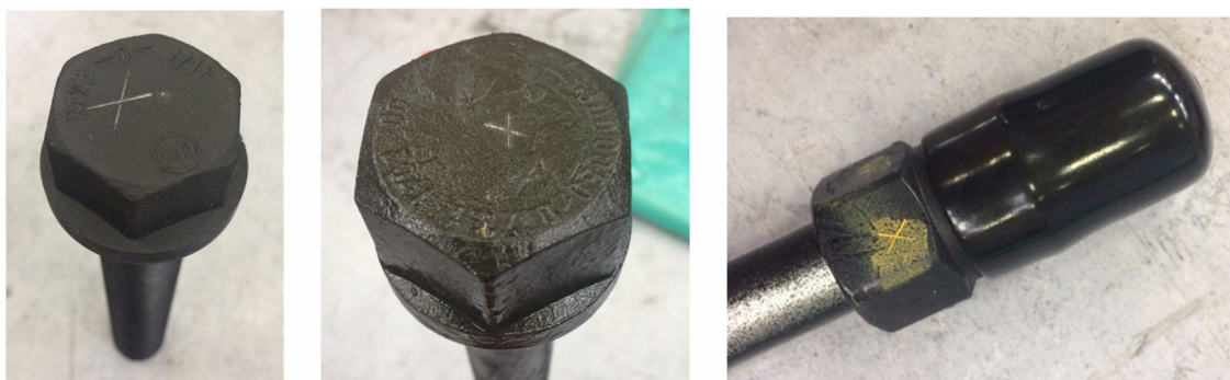
Fig. 115: Examples of markings on screws and HP pipe nut
