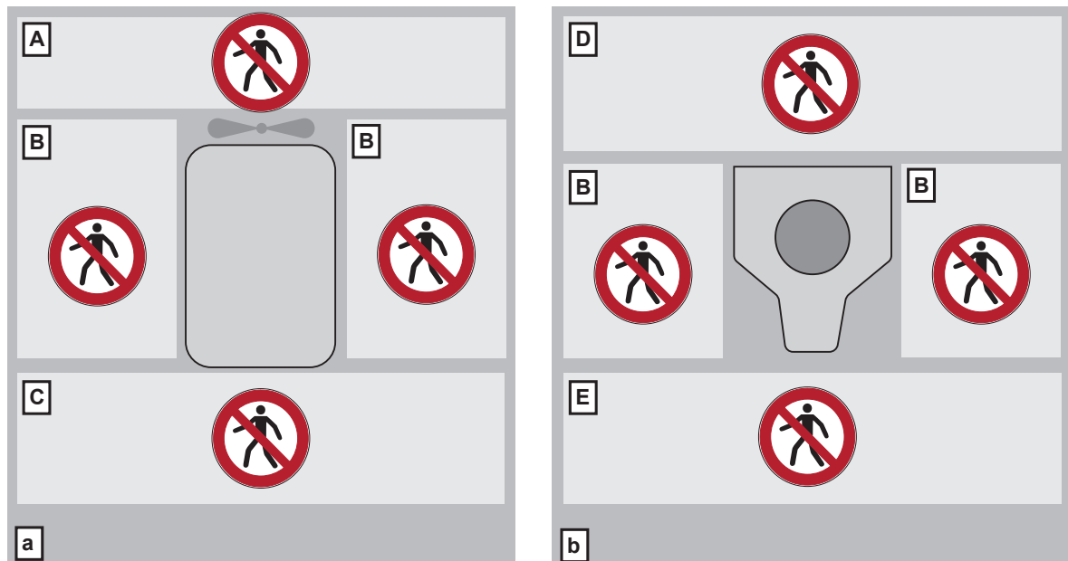
Fig. 20: Safety zones for the engine that is ready for operation or in operation
