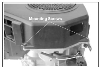
Figure 11-53. Installing Blower Housing.
