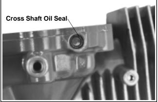
Figure 11-2. Cross Shaft Oil Seal.
