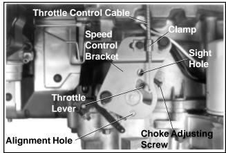
Figure 5-19. Speed Control Bracket Assembly.
