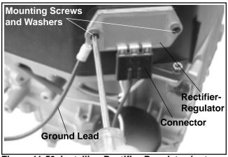
Figure 11-59. Installing Rectifier-Regulator (not on all models).
