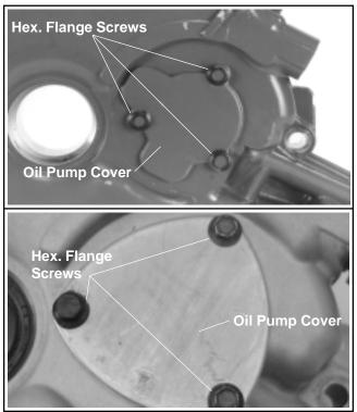
Figure 11-24. Installing Oil Pump Cover.
