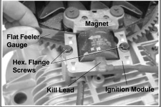
Figure 11-48. Installing Ignition Module.
