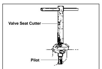
Figure 10-6. Typical Valve Seat Cutter.
