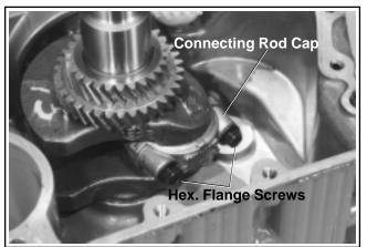
Figure 11-11. Installing Connecting Rod Fasteners.
