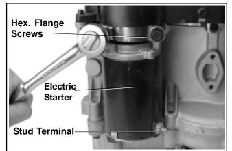
Figure 9-5. Removing Bendix Drive Starter.
