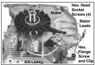
Figure 11-26. Installing Stator.
