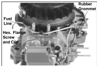
Figure 9-22. Removing Fuel Line (not on all models).
