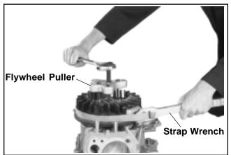
Figure 9-33. Removing Flywheel with a Puller.
