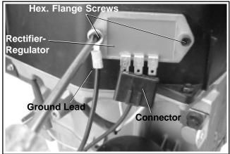
Figure 9-13. Removing Rectifier-Regulator (not on all models).
