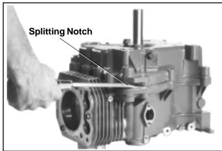
Figure 9-37. Splitting the Oil Pan Crankcase.
