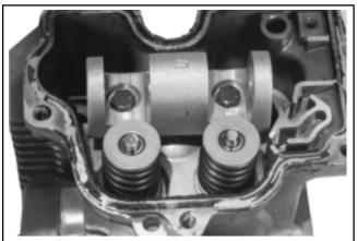
Figure 9-29. Removing Valves. (Bridge Type Head.)
