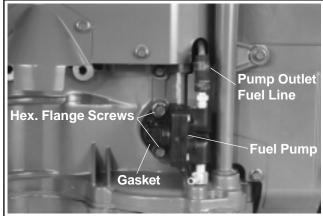
Figure 11-60. Installing Fuel Pump.
