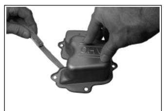
Figure 10-14. Checking with Feeler Gauge.
