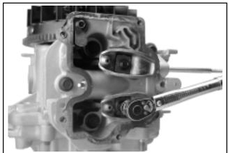
Figure 11-45. Torquing Rocker Arm Mounting Screws.
