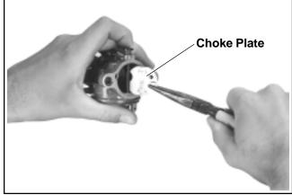
Figure 5-9. Removing Choke Plate.
