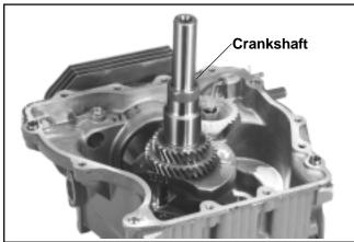
Figure 9-50. Removing Crankshaft.
