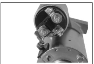
Figure 8-67. Positive Brush Lead Connection.
