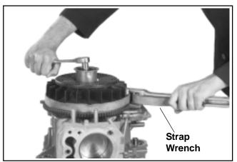
Figure 9-31. Loosening Flywheel Fastener.
