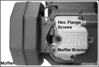
Figure 9-2. Removing Muffler.
