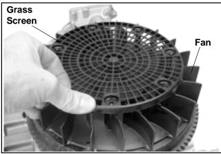
Figure 11-33. Installing Grass Screen (Electric Start Models).
