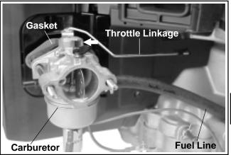
Figure 11-62. Installing Gasket, Carburetor and Fuel Line.
