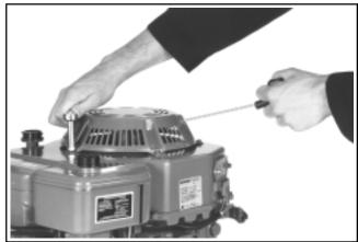
Figure 7-2. Installing Retractable Starter.
