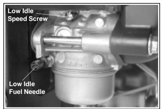
Figure 5-4. Fixed Main Jet Carburetor.
