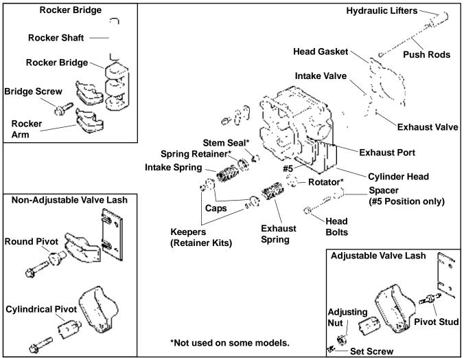
Figure 11-37. Cylinder Head Valve Train Differences.
