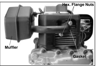
Figure 11-71. Install Muffler.
