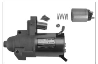
Figure 8-39. Solenoid Removed From Starter.
