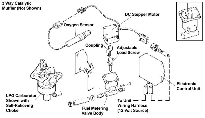
Figure 5-17. Main Components of Kohler Emission Sentry™ System.
