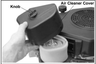
Figure 9-6. Removing Air Cleaner Cover.
