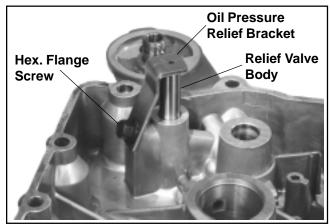
Figure 10-11. Five-Piece Oil Pressure Relief Valve.
