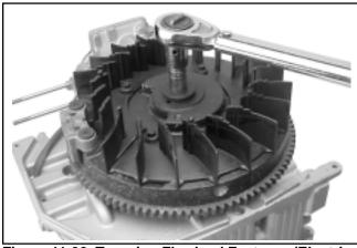
Figure 11-32. Torquing Flywheel Fastener (Electric Start Models).
