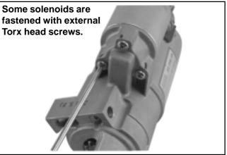
Figure 8-38. Removing Solenoid Screws.
