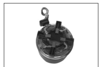
Figure 8-30. Mounting Brush Holder to Frame.
