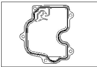
Figure 11-55. Valve Cover Sealant Pattern.
