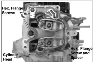
Figure 9-24. Removing Cylinder Head.
