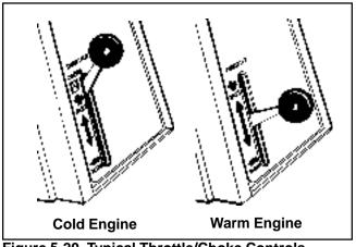
Figure 5-20. Typical Throttle/Choke Controls.
