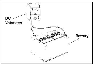
Figure 8-8. Checking Battery Voltage.
