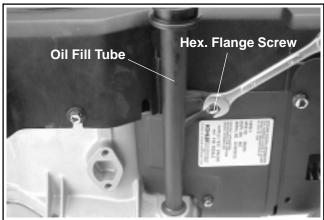
Figure 11-58. Installing Oil Fill Tube.
