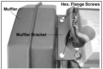
Figure 11-72. Installing Muffler.
