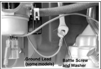
Figure 9-11. Removing Baffle Screw and Washer.
