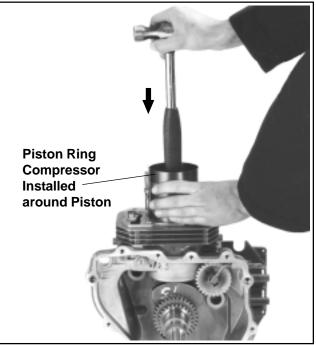
Figure 11-8. Installing Piston and Connecting Rod.
