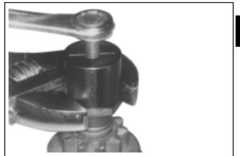
Figure 8-19. Holding Tool and Turning Center Screw (Clockwise) to Remove Retaining Ring.
