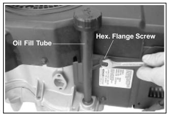
Figure 9-14. Removing Oil Fill Tube.
