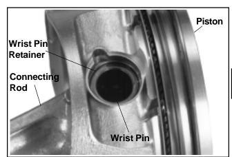
Figure 9-48. Separating Piston from Connecting Rod.
