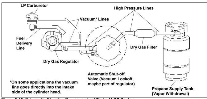
Figure 5-15. Schematic Showing Components of Typical LPG System.
