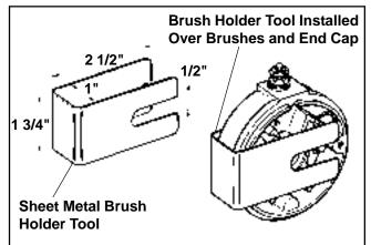
Figure 8-22. Brush Holder Tool (Style "A" End Cap).
