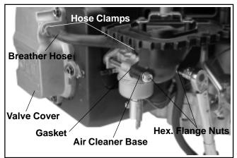
Figure 11-65. Installing Air Cleaner Base.
