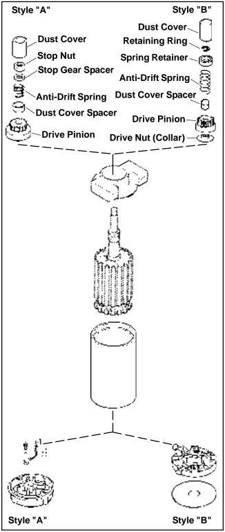
Figure 8-16. Inertia Drive Electric Starter.
