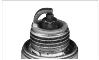
Wet Fouled: A wet plug is caused by excess fuel, or oil in the combustion chamber. Excess fuel could be caused by operating the engine with too much choke or a dirty air filter. Oil in the combustion chamber is usually caused by worn piston rings or valve guides.
