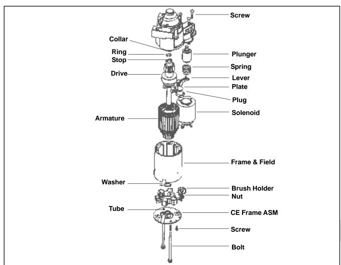
Figure 8-48. Delco-Remy Solenoid Shift Starter.
