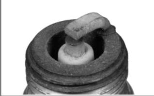
**Normal:** A plug taken from an engine operating under normal conditions will have light tan or gray colored deposits. If the center electrode is not worn, a plug in this condition could be regapped and reused.
