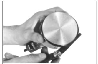
Figure 10-9. Measuring Piston Ring Side Clearance.
