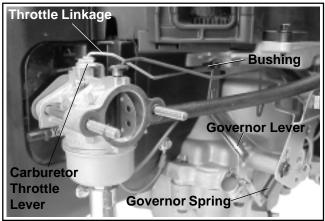
Figure 9-8. Removing Throttle Linkage.
