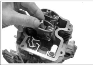
Figure 11-42. Installing Adjustment Nut.
