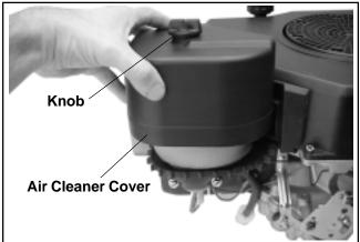
Figure 11-68. Installing Air Cleaner Cover.
