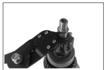
Figure 8-47. Removing Retaining Ring.
