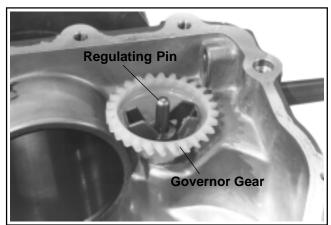
Figure 9-53. Removing Governor Gear.
