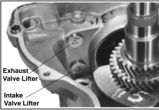
Figure 11-36. Installing Hydraulic Lifters (Camshaft Removed to Show Lifter Positions).
