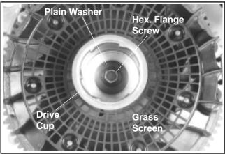
Figure 11-29. Installing Flywheel (Retractable Starter Models).
