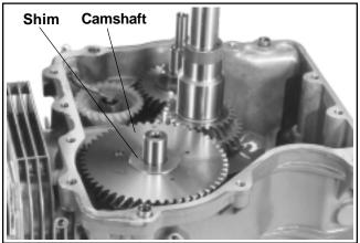
Figure 9-44. Removing Camshaft.
