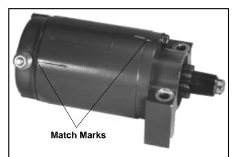
Figure 8-23. Starter Assembly Match Marks.
