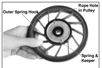
Figure 7-8. Position of Spring and Keeper in Pulley.
