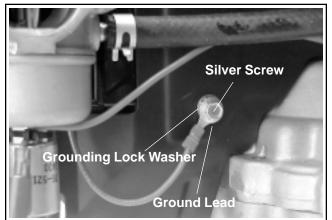
Figure 11-63. Attaching the Ground Lead.
