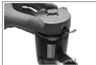
Figure 8-34. Installing End Cap.
