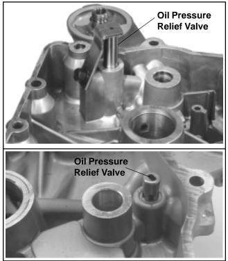
Figure 6-8. Oil Pressure Relief Valve Styles.
