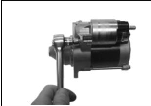
Figure 8-35. Installing Thru Bolts.
