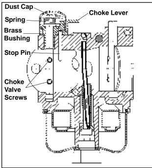
Figure 5-10. Cutaway View Showing Self-Relieving Choke Carburetor.
