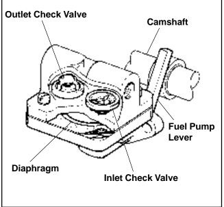
Figure 5-1. Cutaway - Typical Fuel Pump.
