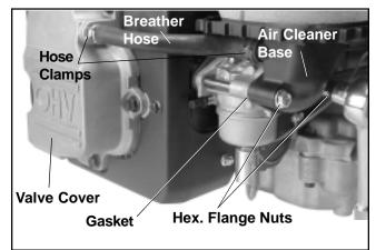
Figure 9-7. Removing Air Cleaner Base.
