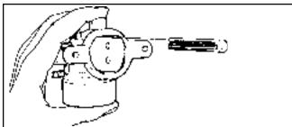
Figure 5-12. Measuring Clearance.
