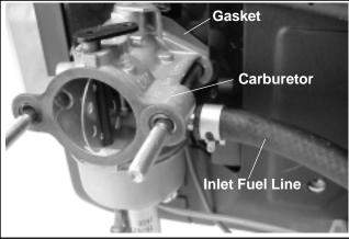
Figure 9-10. Removing Fuel Line and Carburetor.
