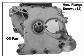
Figure 9-36. Removing Oil Pan.
