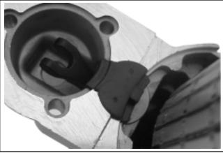
Figure 8-57. Installing Backup Washer and Grommet.
