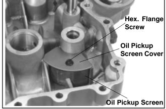
Figure 9-38. Removing Oil Pickup.
