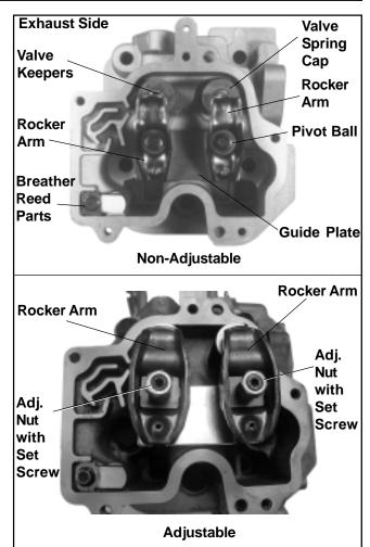
Figure 9-27. Separate Rocker Arm/ Pivot Assembly Style Head.
