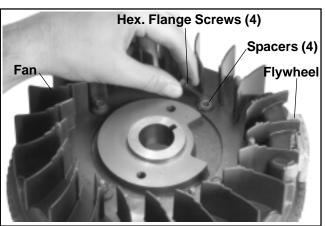
Figure 9-34. Removing Fan from Flywheel.
