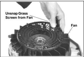
Figure 9-32. Removing Plastic Grass Screen.
