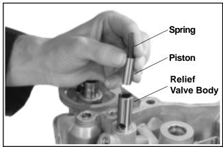
Figure 9-40. Removing Oil Pressure Relief Valve Body, Piston, and Spring (Early Style).
