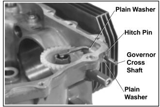
Figure 9-51. Removing Governor Cross Shaft.
