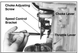
Figure 5-21. Aligning Holes in Speed Control Bracket and Throttle Lever.
