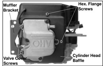
Figure 9-17. Removing Blower Housing and Baffles.
