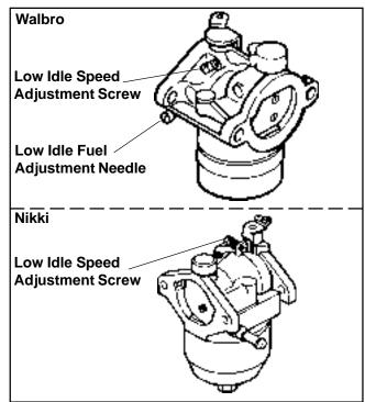
Figure 5-3. Carburetor Adjustment.
