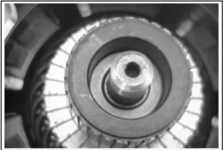
Figure 8-59. Installing Thrust Washer.
