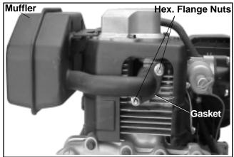
Figure 9-3. Removing Muffler.
