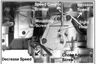
Figure 5-22. Adjusting High Idle Speed.
