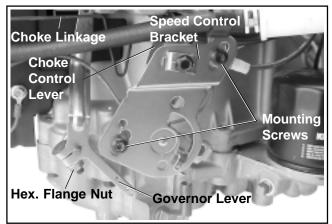
Figure 9-9. Removing Speed Control Bracket.
