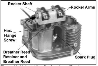
Figure 11-40. Installing Rocker Arms (Rocker Bridge Type).
