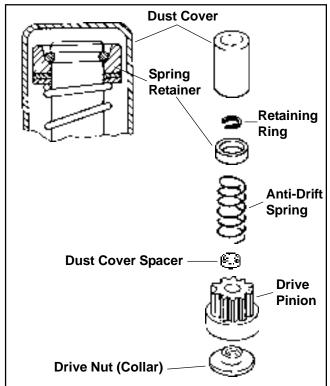
Figure 8-17. Drive Components, "Bonded" Inertia Drive Starter.
