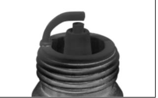
**Carbon Fouled:** Soft, sooty, black deposits indicate incomplete combustion. Incomplete combustion is usually caused by overrich carburetion, weak ignition, or poor compression.
