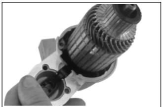
Figure 8-56. Installing Armature and Pivot Lever.
