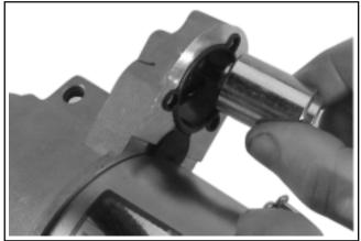
Figure 8-40. Removing Plunger.
