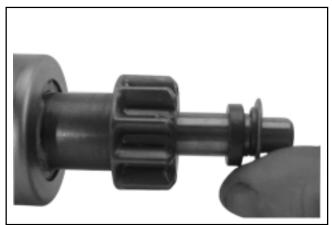
Figure 8-55. Installing Thrust Washer.
