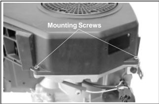
Figure 9-16. Removing Blower Housing and Baffles.
