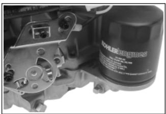
Figure 6-9. Engine Mounted Oil Filter.
