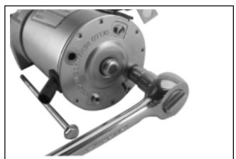
Figure 8-41. Removing Thru Bolts.
