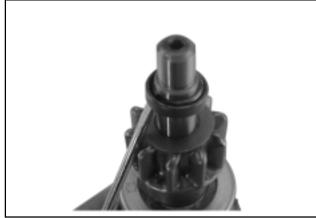
Figure 8-54. Installing Stop Collar and Retainer.
