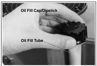
Figure 6-3. Checking Oil Level.
