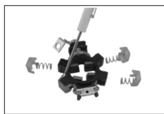
Figure 8-61. Removing Retaining Caps.
