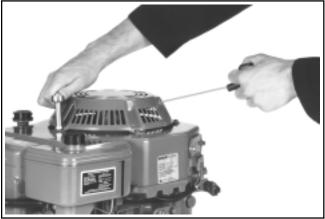
Figure 11-70. Installing Retractable Starter.
