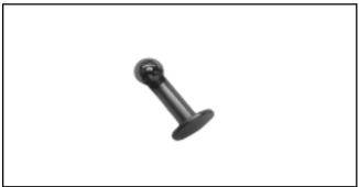
Figure 11-35. Tappet and Ball Bearing Welded Together.
