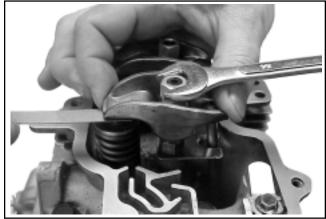
Figure 11-46. Adjusting Valve Lash.
