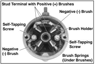
Figure 8-21. Style "A" Commutator End Cap with Brushes.
