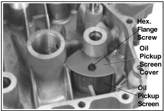
Figure 11-20. Installing Oil Pickup Components.
