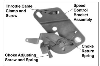
Figure 5-24. Speed Control Bracket Assembly.
