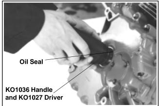
Figure 11-25. Installing Oil Seals.
