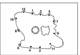
Figure 11-22. Oil Pan Fastener Torque Sequence.
