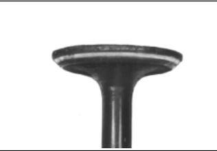
**Overheating:** An exhaust valve subject to overheating will have a dark discoloration in the area above the valve guide. Worn guides and faulty valve springs may cause this condition. Also check for clogged air intake, and blocked fins when this condition is noted.
