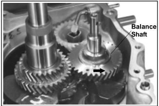
Figure 9-45. Removing Balance Shaft.
