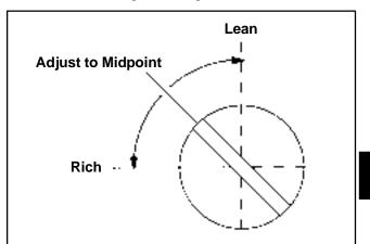
Figure 5-5. Optimum Low Idle Fuel Setting.
