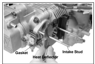
Figure 9-19. Removing Heat Deflector.
