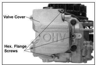
Figure 9-23. Removing Valve Cover.
