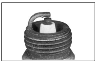
**Chalky White Deposits:** Chalky white-colored deposits indicate overheating. This condition is usually accompanied by excessive gap erosion. A clogged grass screen, clogged cooling fins, and lean carburetion are some causes of overheating.
