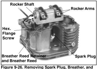
Figure 9-26. Removing Spark Plug, Breather, and Rocker Arms (Rocker Bridge Head).
