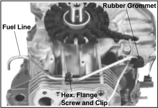
Figure 11-27. Installing Fuel Line.
