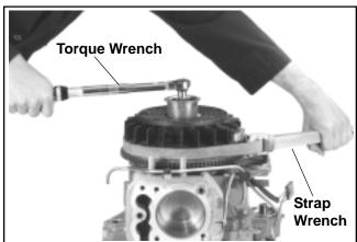
Figure 11-31. Torquing Flywheel Fastener (Retractable Starter Models).
