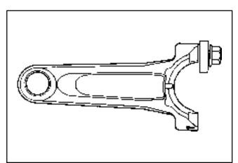
Figure 2-2. Rocker Arm/Crankshaft Tool.
