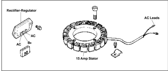
Figure 8-14. 15 amp Stator and Rectifier-Regulator.
