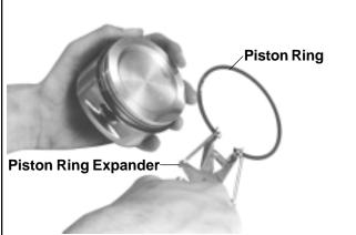
Figure 9-49. Removing Piston Rings.
