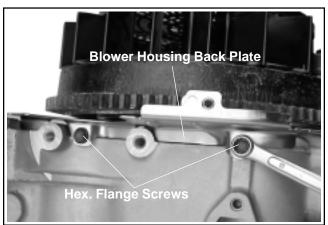
Figure 11-49. Installing Blower Housing Back Plate.
