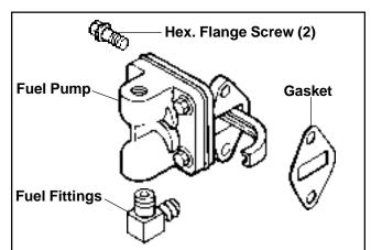
Figure 5-2. Installing Fuel Pump.
