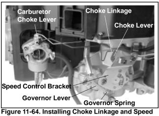
Figure 11-64. Installing Choke Linkage and Speec Control Bracket.
