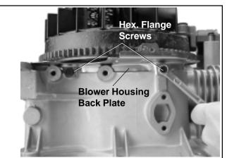
Figure 9-20. Removing Back Plate.
