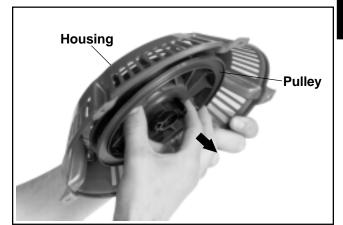
Figure 7-7. Removing Pulley from Housing.
