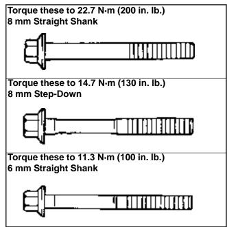
Figure 11-10. Connecting Rod Bolts.
