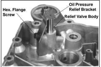
Figure 11-16. Installing Oil Pressure Relief Valve Bracket.
