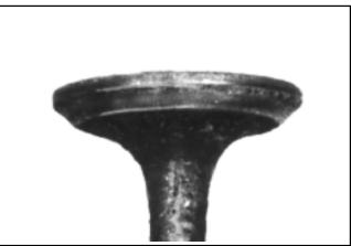
**Stem Corrosion:** Moisture in fuel or from condensation are the most common causes of valve stem corrosion. Condensation occurs from improper preservation during storage and when engine is repeatedly stopped before it has a chance to reach normal operating temperatures. Replace corroded valves.
