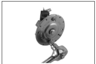
Figure 8-52. Removing Brush Holder.
