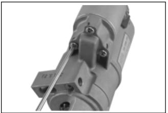
Figure 8-66. Installing Solenoid Screws.
