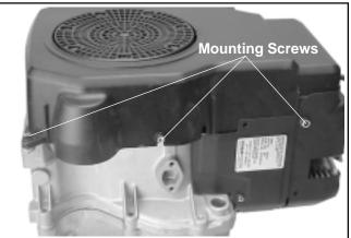
Figure 11-54. Installing Blower Housing.
