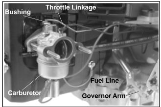
Figure 11-61. Installing Carburetor and External Governor Components.
