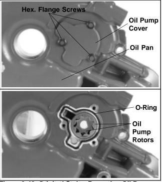
Figure 9-42. Original Style - Removing Oil Pump Covers and Rotors.
