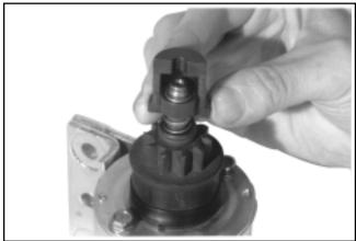
Figure 8-20. Assembling Larger Inner Half Around Spring Retainer.
