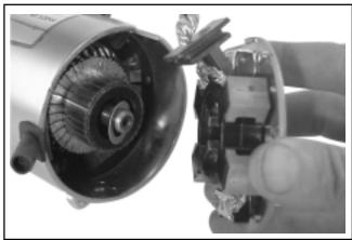
Figure 8-42. Removing Commutator End Plate Assembly.
