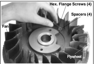
Figure 11-28. Installing Fan to Flywheel.
