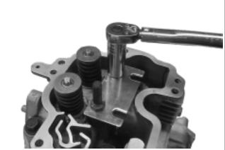
Figure 11-41. Torquing Pivot Studs (Adjustable Valve Lash).
