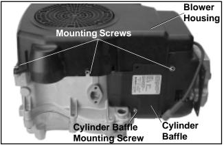
Figure 9-15. Removing Blower Housing and Baffles.
