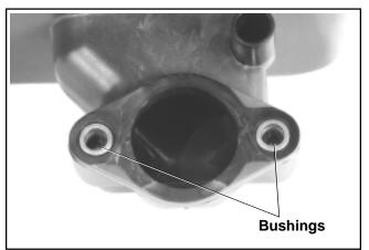
Figure 4-3. Bushings in Air Cleaner Base.
