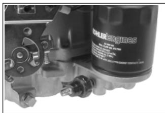
Figure 6-10. Oil Sentry<sup>™</sup> Pressure Switch.\*
