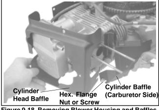
Figure 9-18. Removing Blower Housing and Baffles.
