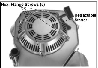
Figure 9-4. Removing Retractable Starter.
