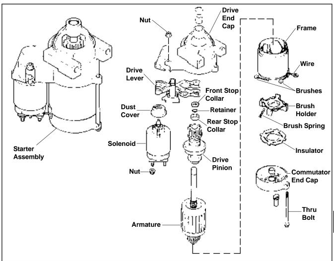
Figure 8-27. Nippendenso Solenoid Shift Starter.
