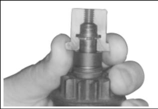
Figure 8-18. Assembling Inner Half of Tool Around Armature Shaft and Retaining Ring.
