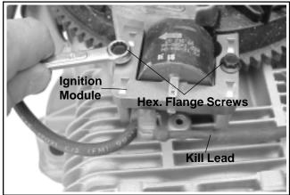
Figure 9-21. Removing Ignition Module.
