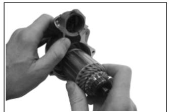
Figure 8-29. Installing Armature.
