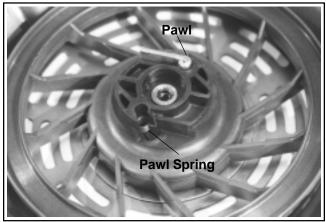
Figure 7-10. Installing Pawls and Pawl Springs.
