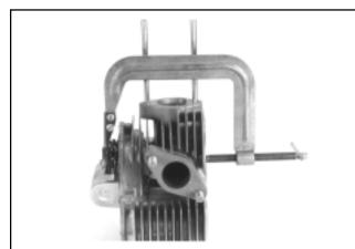
Figure 9-28. Removing Valves with Valve Spring Compressor.
