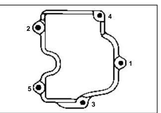
Figure 11-57. Valve Cover Torque Sequence.
