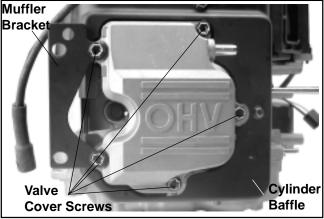
Figure 11-56. Installing Valve Cover (Cast Aluminum Cover Shown).
