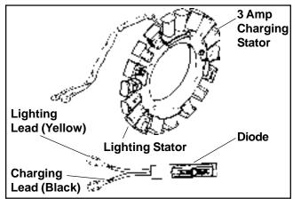
Figure 8-9. 3 amp/70 Watt Stator.
