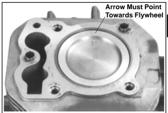
Figure 11-9. Piston Installation Identifier.
