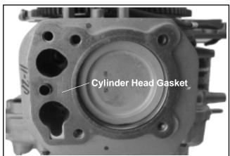
Figure 9-25. Removing Cylinder Head Gasket.
