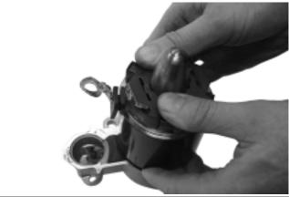
Figure 8-33. Installing Frame with Brush Plate Assembly.
