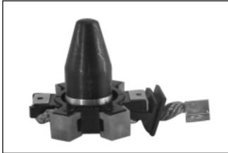
Figure 8-62. Brush Installation Tool with Extension.
