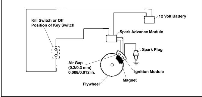
Figure 8-5. Capacitive Discharge Ignition System with Spark Advance.
