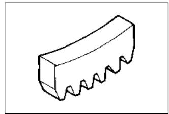
Figure 2-1. Flywheel Holding Tool.
