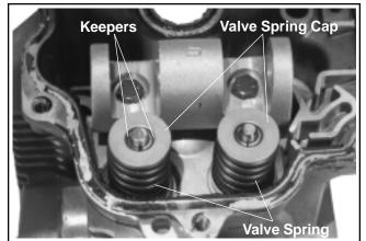
Figure 11-39. Installing Valve Keepers.
