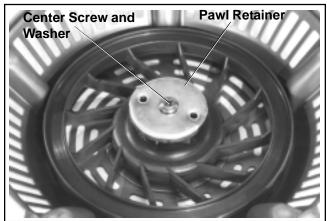
Figure 7-5. Center Screw, Washer and Pawl Retainer.
