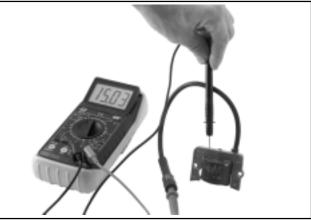
Figure 8-4. Testing Module Secondary.
