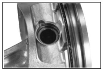
Figure 11-5. Installing Piston to Connecting Rod.
