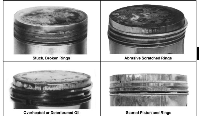
Figure 10-7. Common Types of Piston and Ring Damage.
