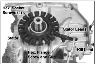
Figure 9-35. Removing Stator.
