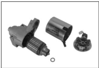
Figure 8-43. Starter Frame Removed.
