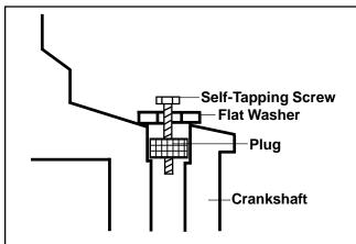
Figure 10-2. Removing Plug.
