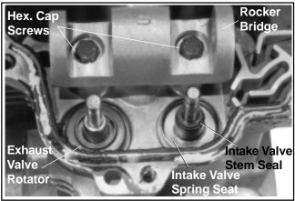
Figure 11-38. Installing Rocker Bridge and Valves.
