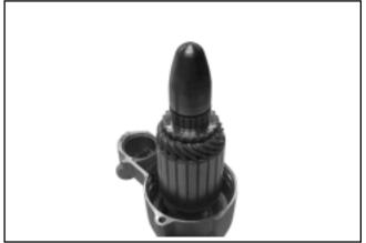
Figure 8-32. Tool on end of Armature.
