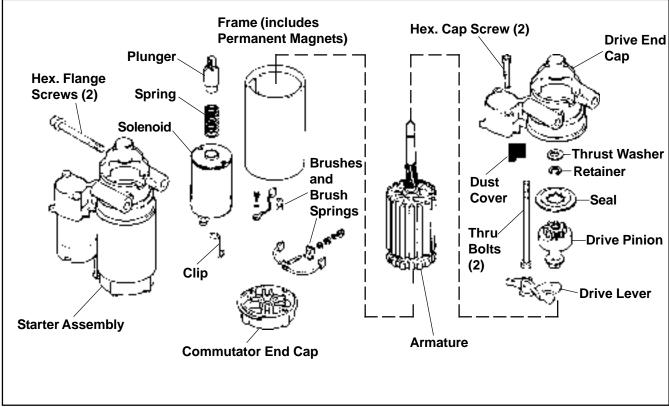
Figure 8-26. UTE Solenoid Shift Electric Starter.
