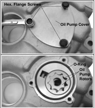
Figure 9-43. New Style - Removing Oil Pump Covers and Rotors.
