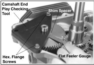
Figure 11-14. Checking Camshaft End Play.
