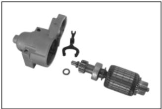
Figure 8-45. Armature and Lever Removed.
