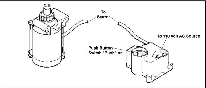
Figure 8-25. 110 Volt UL Approved Electric Starter.
