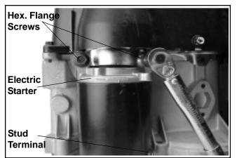
Figure 11-69. Installing Bendix Drive Starter.
