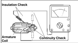
Figure 8-51. Checking Armature.
