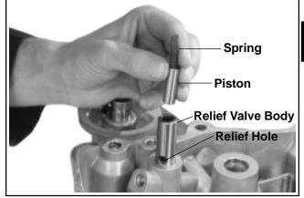
Figure 11-15. Installing Oil Pressure Relief Valve Body, Plunger, and Spring.
