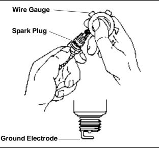
Figure 8-1. Servicing Spark Plug.
