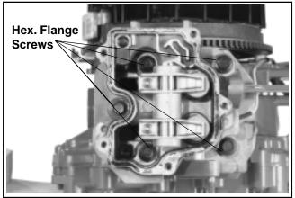
Figure 11-43. Installing Cylinder Head (Rocker Bridge Type Shown).
