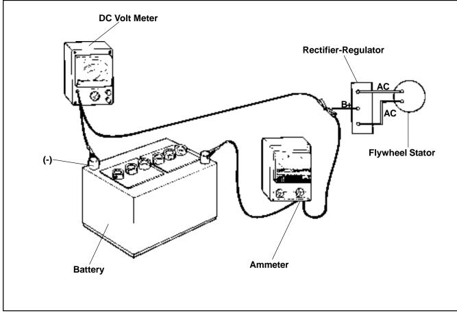
Figure 8-15. Proper Connection to Test 15 amp Charging System.
