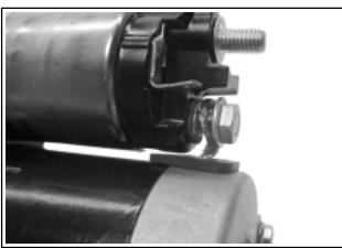
Figure 8-36. Connecting Brush Lead.
