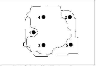
Figure 11-44. Cylinder Head Fastener Torque Sequence.
