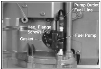
Figure 9-12. Removing Fuel Pump.
