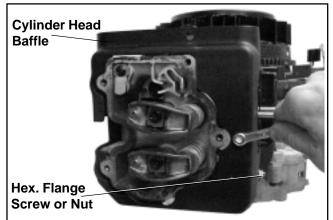
Figure 11-52. Installing Cylinder Head Baffle.
