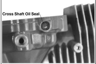
Figure 9-52. Removing Cross Shaft Oil Seal.
