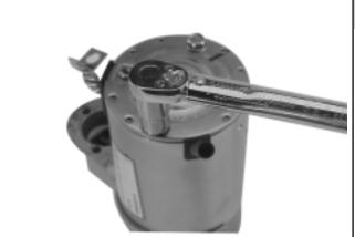
Figure 8-64. Torquing Thru Bolts.
