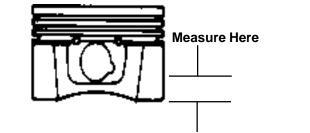
Figure 10-4. Measuring Piston Diameter.
