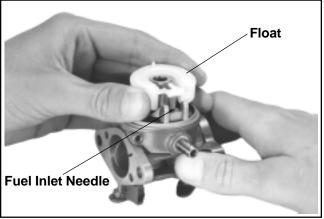
Figure 5-14. Installing Float and Fuel Inlet Needle.
