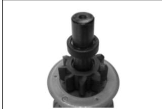
Figure 8-28. Lock Collar around Retaining Ring.
