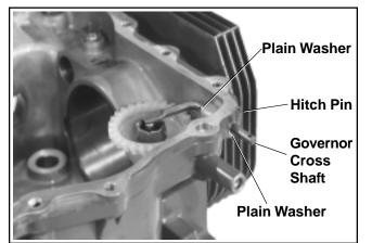
Figure 11-3. Installing Cross Shaft.
