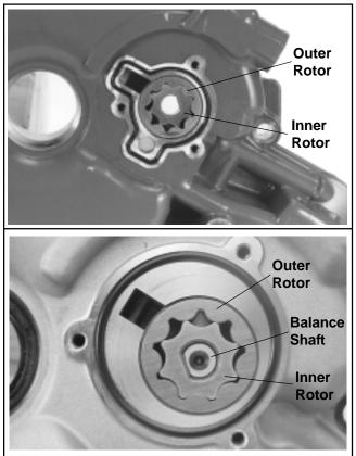
Figure 11-23. Installing Oil Pump Gears and O-Ring.
