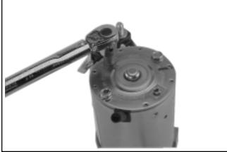
Figure 8-65. Torquing Brush Holder Screws.
