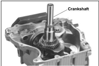
Figure 11-4. Installing Crankshaft.
