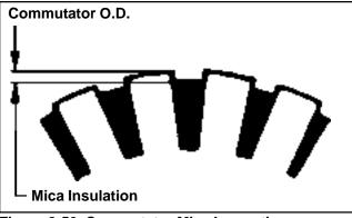
Figure 8-50. Commutator Mica Inspection.
