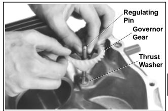
Figure 11-1. Installing Governor Gear.
