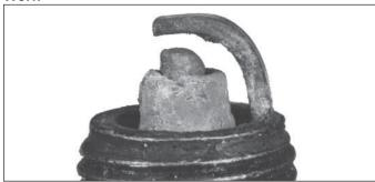
On a worn plug, center electrode will be rounded and gap will be greater than specified gap. Replace a worn spark plug immediately.
