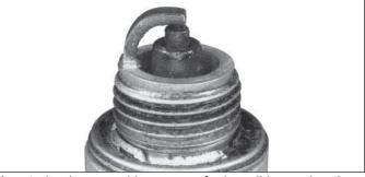
A wet plug is caused by excess fuel or oil in combustion chamber. Excess fuel could be caused by a restricted air cleaner or a fuel mixture problem. Oil in combustion chamber is usually caused by a restricted air cleaner, a breather problem, worn piston rings, or valve guides.
