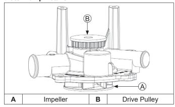
Water/coolant pump consists of a sealed impeller assembly, which includes outer cover and a cogged drive pulley. When pump is mounted to crankcase, impeller fits into a cast recess, and cover seals against an O-ring outside perimeter of recess.
