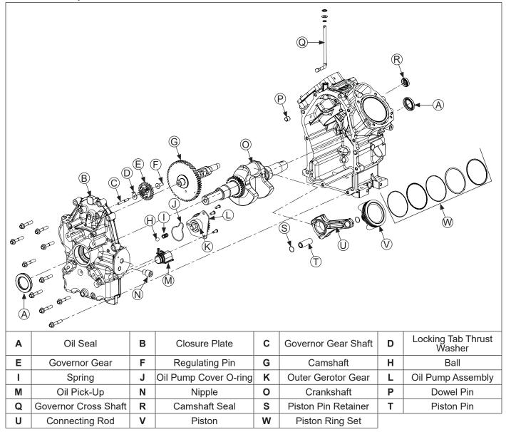
NOTE: Make sure engine is assembled using all specified torque values, tightening sequences and clearances. Failure to observe specifications could cause severe engine wear or damage. Always use new gaskets. Apply a small amount of oil to threads of critical fasteners before assembly, unless a Sealant or Loctite® is specified or preapplied.
