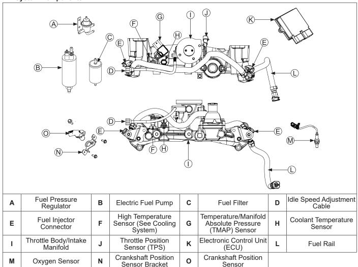
Typical electronic fuel injection (EFI) system and related components include:
