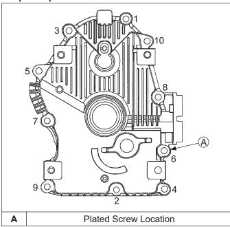
RTV silicone sealant is used as a gasket between closure plate and crankcase. Always use fresh sealant. Using outdated sealant can result in leakage.
