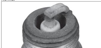
Plug taken from an engine operating under normal conditions will have light tan or gray colored deposits. If center electrode is not worn, plug can be set to proper gap and reused.
