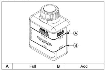
NOTE: Do not operate engine without coolant in system.
