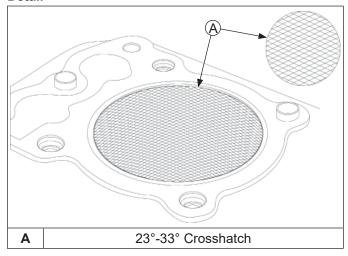
While most commercially available cylinder hones can be used with either portable drills or drill presses, use of a low speed drill press is preferred as it facilitates more accurate alignment of bore in relation to crankshaft crossbore. Honing is best accomplished at a drill speed of about 250 RPM and 60 strokes per minute. After installing coarse stones in hone, proceed as follows:
