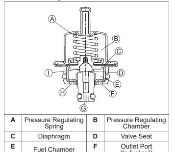
Regulator is a sealed, non-serviceable assembly. If it is faulty, it must be replaced as follows:
