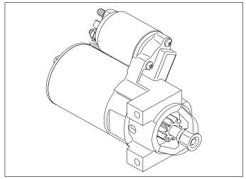
When power is applied to starter electric solenoid moves drive pinion out onto drive shaft and into mesh with flywheel ring gear. When pinion reaches end of drive shaft it rotates flywheel and cranks engine.
