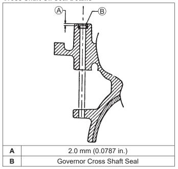
Remove governor cross shaft oil seal from crankcase and replace it with a new one if seal is damaged and/ or leaks. Install new seal to depth shown using a seal installer.
