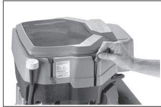
Figure 8. Unhooking Retaining Straps.
