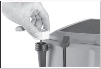
Figure 5. Checking Oil Level.
