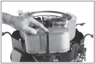
Figure 21. Unhooking Retaining Strap.
