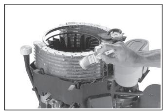
Figure 22. Clean Radiator Cooling Fins.
