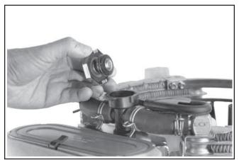
Figure 11. Removing Radiator Cap.
