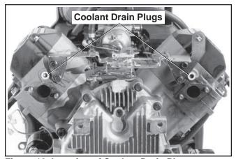
Figure 12. Location of Coolant Drain Plugs.
