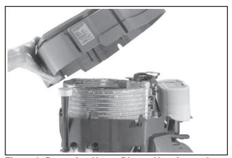
Figure 9. Removing Upper Blower Housing and Screen Assembly.
