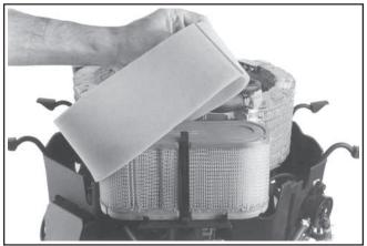
Figure 17. Removing Precleaner from Paper Element.
