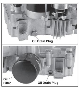
Figure 7. Oil Drain Plugs and Oil Filter.
