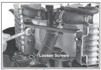
Figure 13. Loosening Screws.
