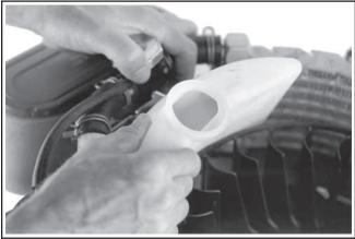
Figure 15. Removing Reservoir.
