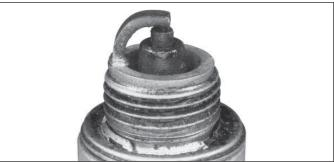
A wet plug is caused by excess fuel or oil in combustion chamber. Excess fuel could be caused by a restricted air cleaner, a throttle body problem, or operating engine with too much choke. Oil in combustion chamber is usually caused by a restricted air cleaner, a breather problem, worn piston rings, or valve guides.
