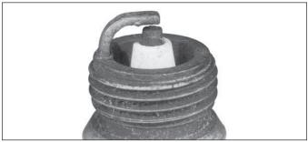
Chalky, white deposits indicate very high combustion temperatures. This condition is usually accompanied by excessive gap erosion. Lean throttle body settings, an intake air leak, or incorrect spark timing are normal causes for high combustion temperatures.
