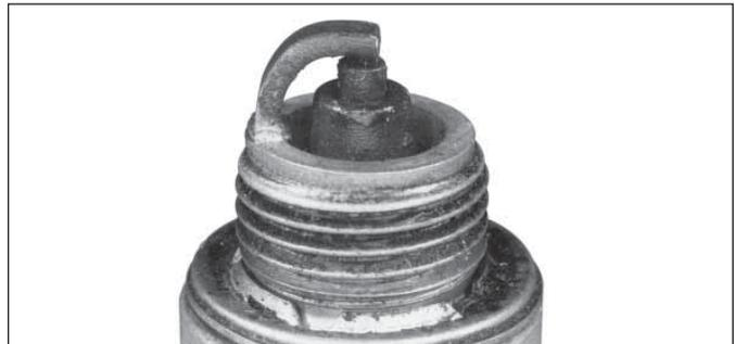
A wet plug is caused by excess fuel or oil in combustion chamber. Excess fuel could be caused by a restricted air cleaner, a throttle body problem, or operating engine with too much choke. Oil in combustion chamber is usually caused by a restricted air cleaner, a breather problem, worn piston rings, or valve guides.
