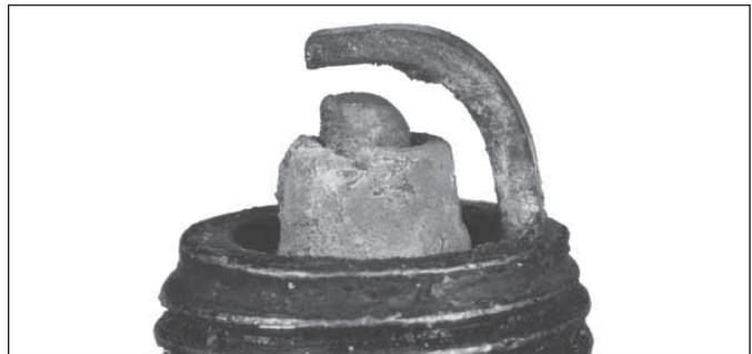
On a worn plug, center electrode will be rounded and gap will be greater than specified gap. Replace a worn spark plug immediately.
