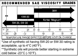
Figure 3. Viscosity Grades Table.
