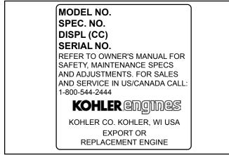
Figure 2. Engine Identification Label.
