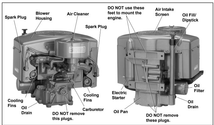
Figure 1. Typical Magnum Vertical Shaft Engine.
