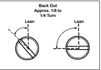
Figure 10. Optimum Low Idle Fuel Setting.
