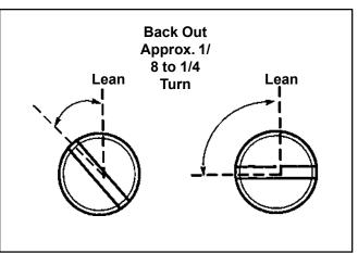
Figure 9. Optimum Main Fuel Setting.
