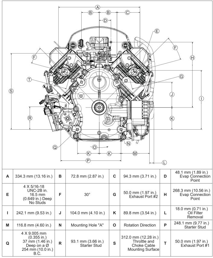
Engine Dimensions with Low Profile, High Performance, or PRO Performance Air Cleaner-Starter Side
