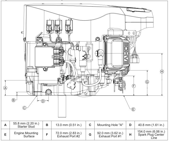
Engine Dimensions with Low Profile, High Performance, or PRO Performance Air Cleaner-Valve Cover Side **B** E (D) (C)
