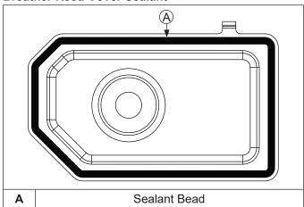
NOTE: RTV sealant should be allowed to cure a minimum of 1 hour before engine is started.
