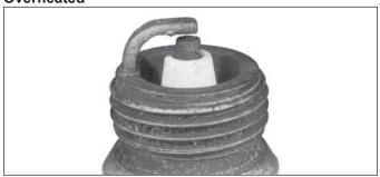
Chalky, white deposits indicate very high combustion temperatures. This condition is usually accompanied by excessive gap erosion. Lean fuel mixture settings, an intake air leak, or incorrect spark timing are normal causes for high combustion temperatures.
