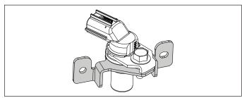
A sealed, non-serviceable assembly. If fault code P0337 is present and engine does not start/run, proceed to step 1. If P0337 is present and engine operates, clear codes and retest. If Fault Code diagnosis indicates a problem within this area, test and correct as follows.
