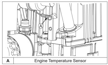
NOTE: Engine temperature sensor resembles a ground wire.
