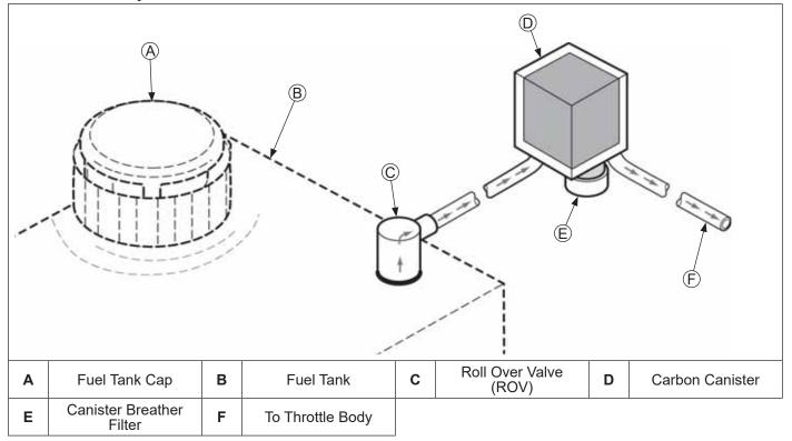
For equipment to be Tier III compliant, it may be fitted with a Kohler supplied canister vapor recovery system, or a system developed and installed by Original Equipment Manufacturer (OEM). Details on Kohler system are included below.
