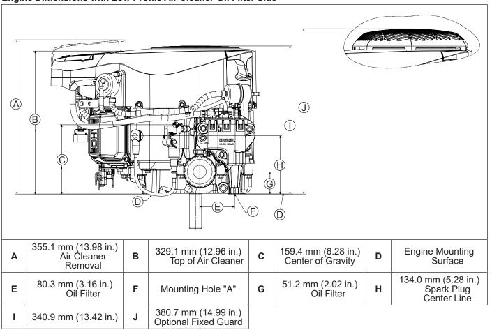
**Engine Dimensions with Low Profile or High Performance Air Cleaner-Engine Mounting Surface (PTO End)**
