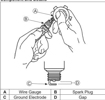
NOTE: Do not clean spark plug in a machine using abrasive grit. Some grit could remain in spark plug and enter engine causing extensive wear and damage.
