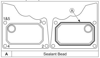
NOTE: Always use fresh sealant. Using outdated sealant can result in leakage. Refer to Tools and Aids for a listing of approved sealants.
