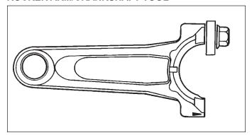
A spanner wrench to lift rocker arms or turn crankshaft may be made out of an old junk connecting rod.
