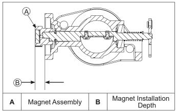
Magnet assembly is captured in a small plastic housing that is press fit to end of throttle shaft. This generally does not need replacement. If replacement is required, it can be replaced as follows:
