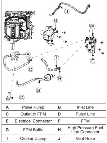
NOTE: Do not cut Oetiker clamp unless fuel line or FPM are being replaced.
