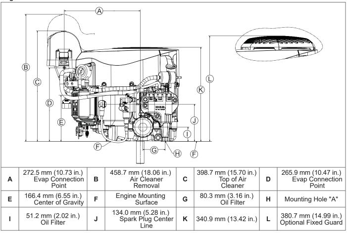
**Engine Dimensions with PRO Performance Air Cleaner-Engine Mounting Surface (PTO End)**
