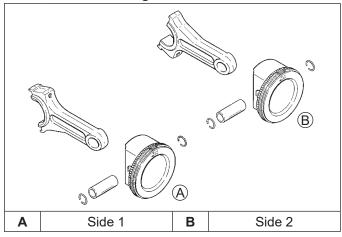
NOTE: Cylinders are numbered on crankcase. Make sure to install piston, connecting rod, and end cap into its appropriate cylinder bore as previously marked during disassembly. Do not mix end caps and connecting rods.
