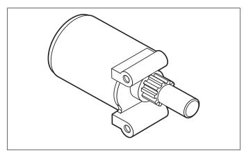
When power is applied to starter, armature rotates. As armature rotates, drive pinion moves out on drive shaft splines and into mesh with flywheel ring gear. When pinion reaches end of drive shaft, it rotates flywheel and cranks engine.
