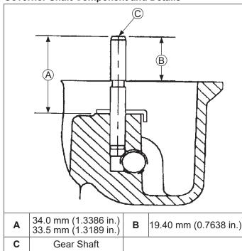
NOTE: Governor gear is held onto shaft by small molded tabs in gear. When gear is removed from shaft, these tabs are destroyed and gear must be replaced. Therefore, remove gear only if absolutely necessary.
