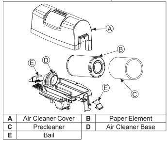
NOTE: Operating engine with loose or damaged air cleaner components could cause premature wear and failure. Replace all bent or damaged components.
