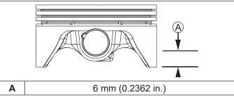
NOTE: Do not use a feeler gauge to measure piston-tobore clearance, it will yield inaccurate measurements. Always use a micrometer.
