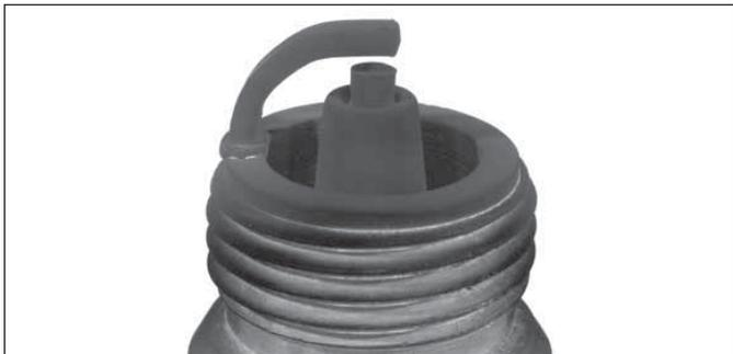
Soft, sooty, black deposits indicate incomplete combustion caused by a restricted air cleaner, over rich carburetion, weak ignition, or poor compression.
