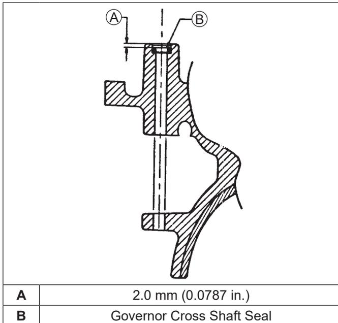
If governor cross shaft seal is damaged and/or leaks, replace it using these following procedures.
