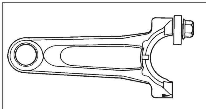
A spanner wrench to lift rocker arms or turn crankshaft may be made out of an old junk connecting rod.
