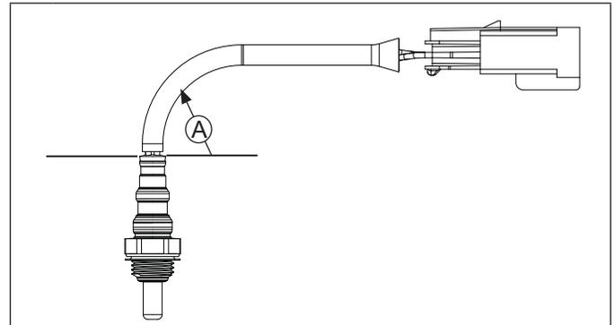
**A** Keep a minimum of 25 mm (1.0 in.) radius at grommet.
