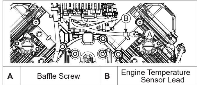
1. Remove screw securing inner baffle and engine temperature sensor lead.
