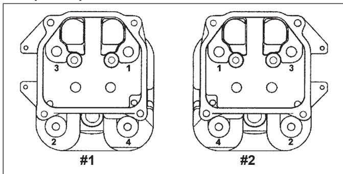
NOTE: Cylinder heads must be attached with original type of mounting hardware, using either screws, or mounting studs with nuts and washers. Do not intermix components.
