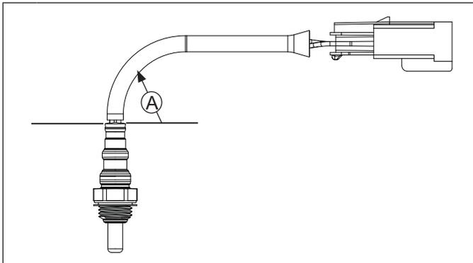
**A** Keep a minimum of 25 mm (1.0 in.) radius at grommet.
