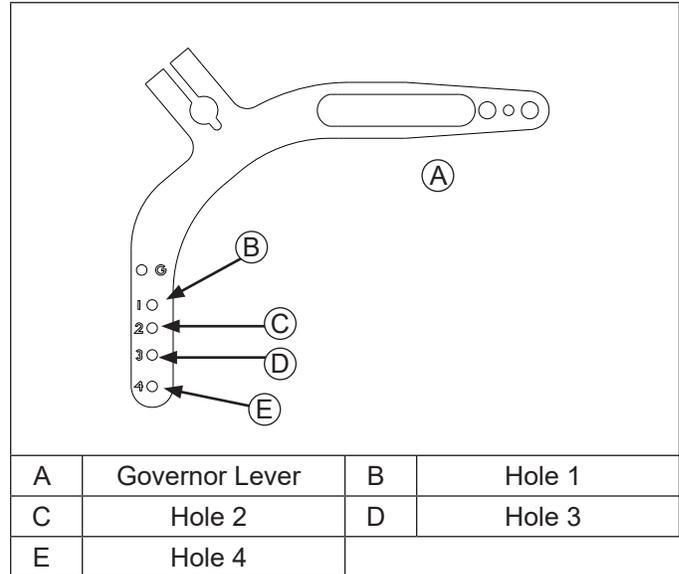
Governor sensitivity is adjusted by repositioning governor spring in holes of governor lever. If speed surging occurs with a change in engine load, governor is set too sensitive. If a big drop in speed occurs when normal load is applied, governor should be set for greater sensitivity. Adjust as follows:
