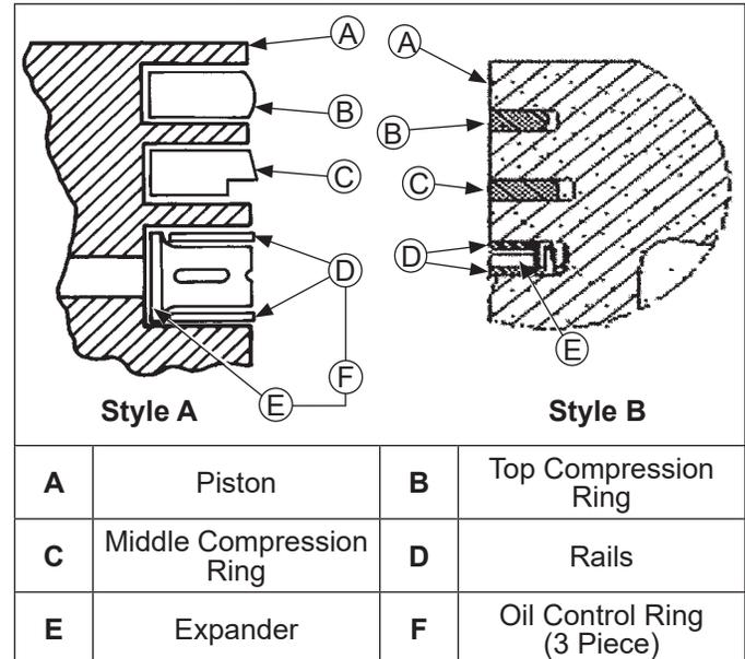
**NOTE:** Rings must be installed correctly. Ring installation instructions are usually included with new ring sets. Follow instructions carefully. Use a piston ring expander to install rings. Install bottom (oil control) ring first and top compression ring last.
