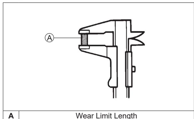
Inspect both springs and brushes for wear, fatigue, or damage. Measure length of each brush. Minimum length for each brush is 7.6 mm (0.300 in.). Replace brushes if they are worn, undersize, or condition is questionable.
