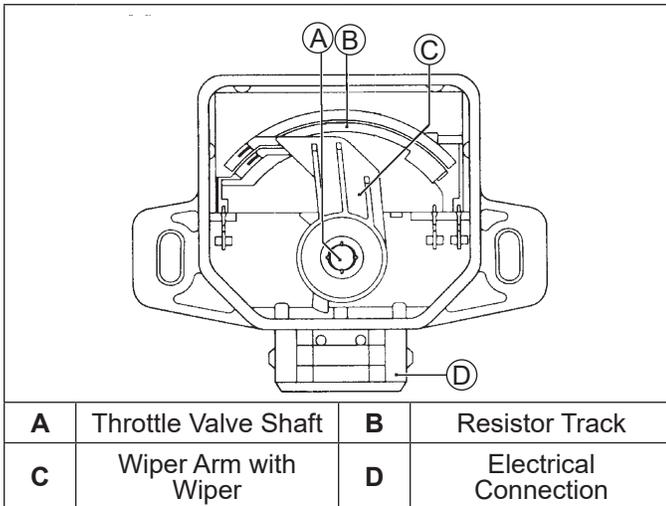
The TPS is a sealed, non-serviceable assembly. If diagnosis indicates a bad sensor, complete replacement is necessary. If a blink code indicates a problem with TPS, it can be tested as follows:
