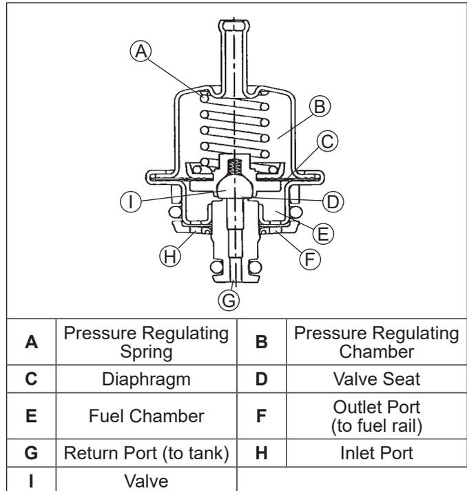
Depending on application, regulator may be located in fuel tank along with fuel pump, or outside tank just down line from pump. Regulator is a sealed, non-serviceable assembly. If it is faulty, it must be separated from base/holder assembly and replaced as follows:
