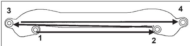
1. Install intake manifold and new gaskets, with wiring harness attached, to cylinder heads. Slide any wiring harness clips onto appropriate bolts before installing. Make sure gaskets are in proper orientation. Torque screws in 2 stages, first to 7.8 N·m (69 in. lb.), then to 10.5 N·m (93 in. lb.), using sequence shown.
