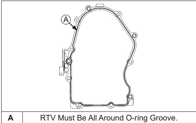
**A** RTV Must Be All Around O-ring Groove.
