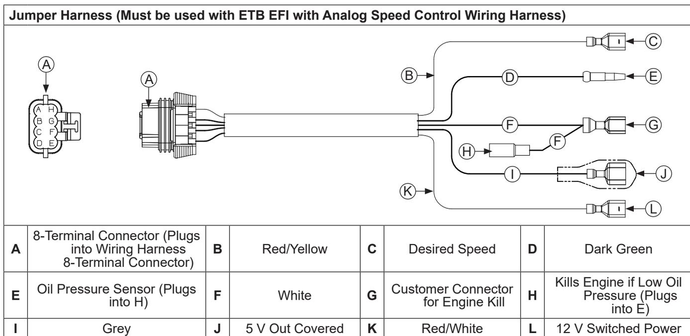
Engines equipped with this jumper harness feature ETB-Analog speed control. Engine speed is adjusted using variable voltage inputs received by ECU from OEM controller.
