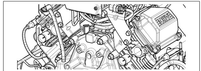
1. Install port liners (if equipped), slotted end first, into exhaust ports until finger tight. (Exhaust components will press them to final depth.) Install exhaust gaskets and muffler on exhaust studs.
