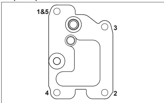
1. Be sure sealing surfaces of crankcase and breather cover are clean of old gasket material. Do not scrape surfaces as this could result in leakage. Use a new gasket when installing breather cover.
