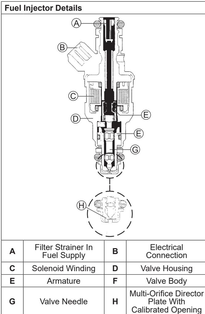
Injector problems typically fall into three general categories: electrical, dirty/clogged, or leakage. An electrical problem usually causes one or both of injectors to stop functioning. Several methods may be used to check if injectors are operating.
