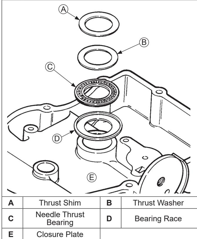
Some specifications use a needle type thrust bearing, thrust washer and shim spacer to control end play of crankshaft. If these items are noted during disassembly, make sure they are reinstalled in sequence shown. A different procedure will have to be followed to check and adjust crankshaft end play on these models.
