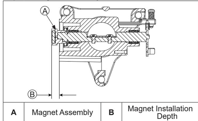
Magnet assembly is captured in a small plastic housing that is press fit to end of throttle shaft. This generally does not need replacement. If replacement is required, can be replaced as follows:
