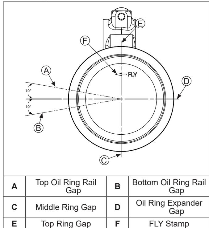
NOTE: Rings must be installed correctly. Ring installation instructions are usually included with new ring sets. Follow instructions carefully. Use a piston ring expander to install rings. Install bottom (oil control) ring first and top compression ring last.
