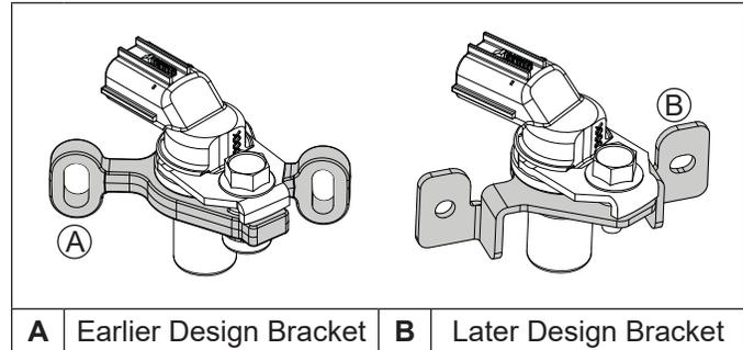
Crankshaft position sensor is essential to engine operation; constantly monitoring rotation and speed (RPM) of crankshaft. There are 23 consecutive teeth cast into flywheel. One tooth is missing and is used to reference crankshaft position for ECU. Inductive crankshaft position sensor with earlier design bracket is mounted 0.20-0.70 mm (0.008-0.027 in.) from flywheel. Later design bracket requires no adjustment.
