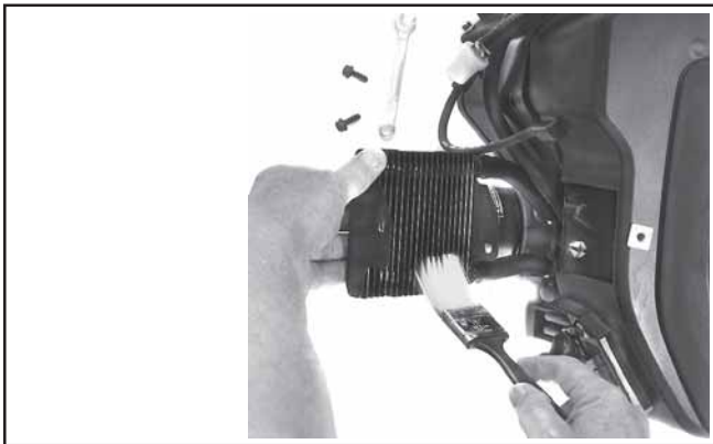
Figure 10. Cleaning Oil Cooler.
