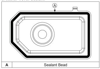
NOTE: RTV sealant should be allowed to cure a minimum of 1 hour before engine is started.
