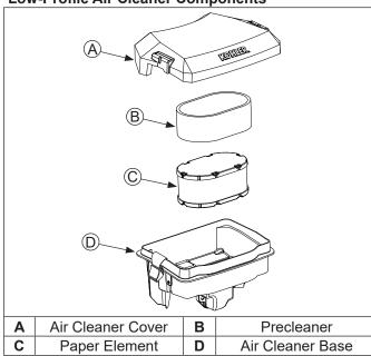
NOTE: Operating engine with loose or damaged air cleaner components could cause premature wear and failure. Replace all bent or damaged components.
