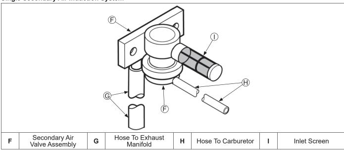
For engine to be Tier III compliant, it may be fitted with a secondary air induction system (SAI).
