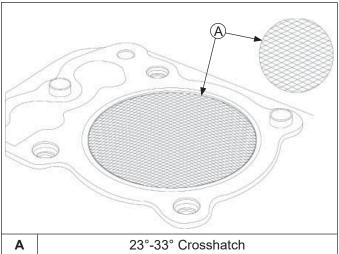
NOTE: Kohler pistons are custom-machined to exacting tolerances. When over-sizing a cylinder, it should be machined exactly 0.25 mm (0.010 in.) over new diameter (refer to Specifications). Oversize Kohler replacement piston will then fit correctly.
