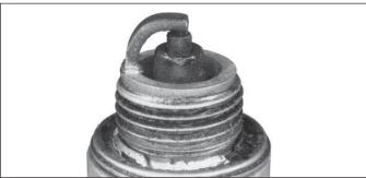
A wet plug is caused by excess fuel or oil in combustion chamber. Excess fuel could be caused by a restricted air cleaner, a carburetor problem, or operating engine with too much choke. Oil in combustion chamber is usually caused by a restricted air cleaner, a breather problem, worn piston rings, or valve guides.
