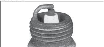
Chalky, white deposits indicate very high combustion temperatures. This condition is usually accompanied by excessive gap erosion. Lean carburetor settings, an intake air leak, or incorrect spark timing are normal causes for high combustion temperatures.
