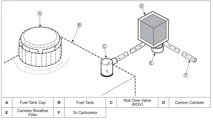
For engine to be Tier III compliant, it may be fitted with a Kohler supplied canister vapor recovery system, or a system developed and installed by Original Equipment Manufacturer (OEM). Details on Kohler system are included below.
