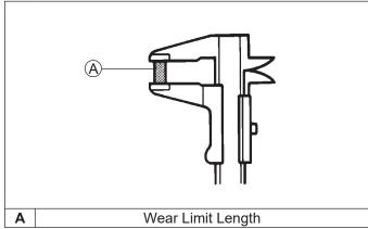
Inspect both springs and brushes for wear, fatigue, or damage. Measure length of each brush. Minimum length for each brush is 7.6 mm (0.300 in.). Replace brushes if they are worn, undersize, or condition is questionable.
