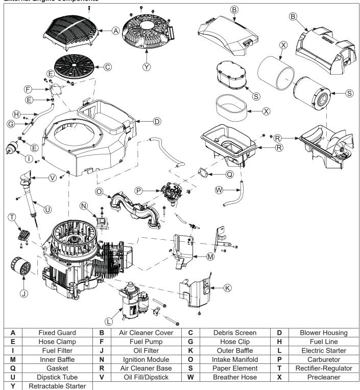
Clean all parts thoroughly as engine is disassembled. Only clean parts can be accurately inspected and gauged for wear or damage. There are many commercially available cleaners that will quickly remove grease, oil and grime from engine parts. When such a cleaner is used, follow manufacturer's instructions and safety precautions carefully.
