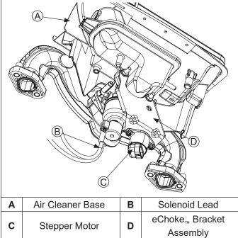
NOTE: On engines equipped with eChoke, stepper motor has a special retract routine that can be activated to ensure motor is in correct position prior to removal or upon replacement of stepper motor when a problem is shown to exist with stepper motor assembly and carburetor.
