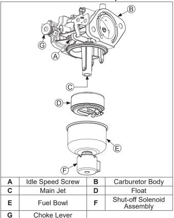
Engines in this series are equipped with either a Keihin or Walbro fixed main jet carburetor. Most carburetors utilize a fuel shut-off solenoid and feature a self-relieving choke.
