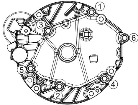
Valve Cover Fasteners
