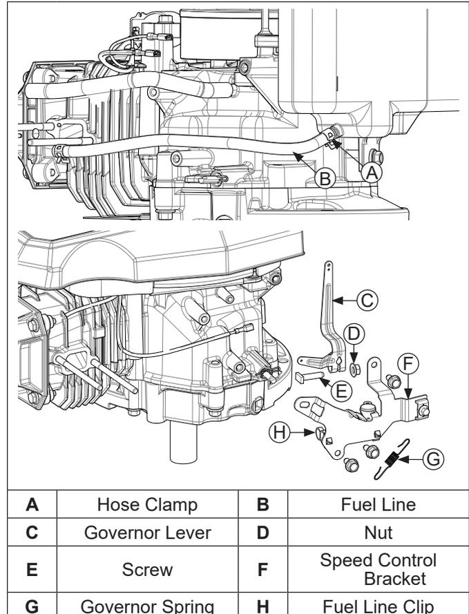
**NOTE:** Fuel line connecting carburetor and fuel tank is held in place by plastic fuel line clips, mounted on back of speed control bracket. If bracket is removed from crankcase, it will remain attached to fuel hose. Should replacement of speed control bracket be required, disconnect fuel line from fuel filter or carburetor and slide bracket off hose. Do not disconnect fuel hose from fuel tank.
