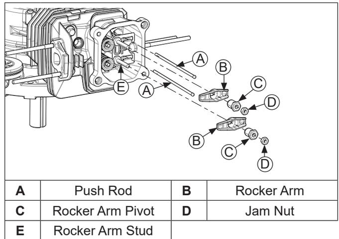
NOTE: Installation and seating of push rods into tappet recesses during this sequence is critical. To aid with proper installation of push rods and rocker arms, and for adjusting valve lash, position engine with cylinder head up. When properly installed, push rods extend approximately 1 in. (25.4 mm) above guide plate.
