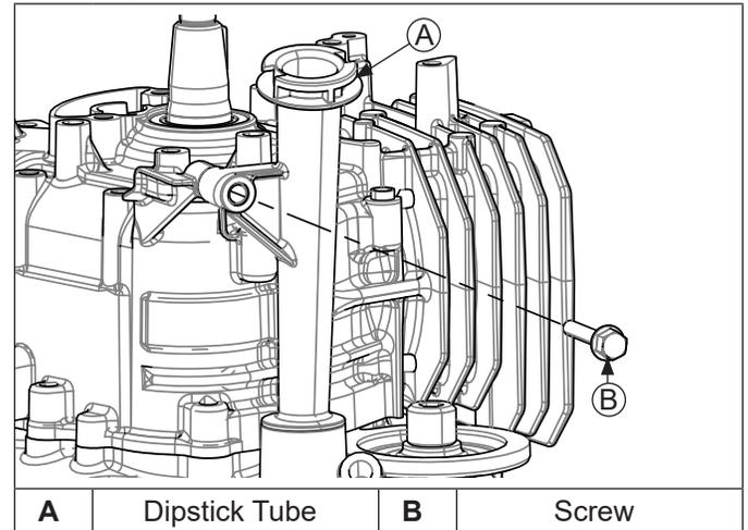
Insert dipstick tube into oil pan and secure to crankcase with screw. Torque screw to 8 N·m (71 in. lb.).
