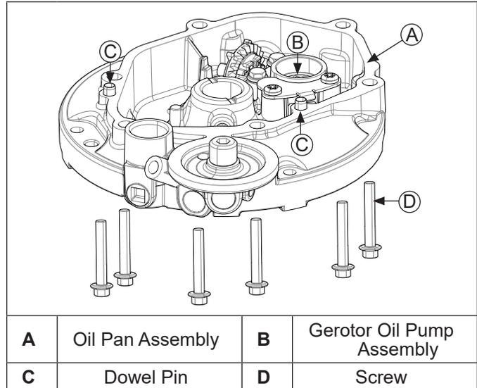
NOTE: Oil pan is sealed to crankcase using RTV silicone sealant. When removing oil pan, use care to not damage sealing surface of crankcase.
