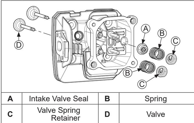
1. Install intake and exhaust valves into their respective positions in cylinder head.
