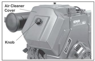
Figure 9. Air Cleaner Housing Components.
