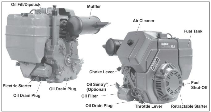
Figure 1. Typical Command Horizontal Shaft Engine.
