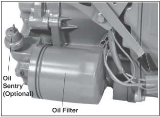
Figure 8. Oil Filter and Optional Oil Sentry Switch.
