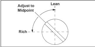
Figure 14. Optimum Low Idle Fuel Setting.
