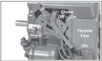
Figure 5. Throttle and Choke Positions for Starting Engine.
