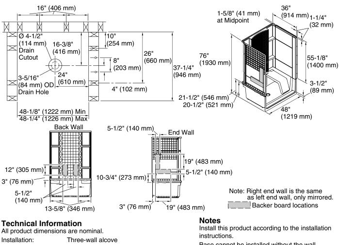
Drain location:CenterMinimum flat for door:3-1/4" (83 mm)Threshold height:3-1/2" (89 mm)Maximum door height:70-5/8" (1794 mm)Maximum door width:44-5/8" (1133 mm)
