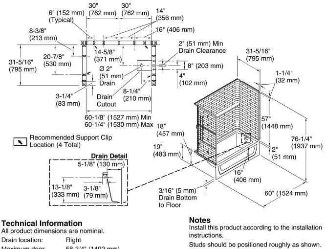
Maximum door 58-3/4" (1492 mm) height: Maximum door 57-5/8" (1464 mm) width: Studs should be positioned roughly as shown. Double studding is recommended for pivot shower door installations.
