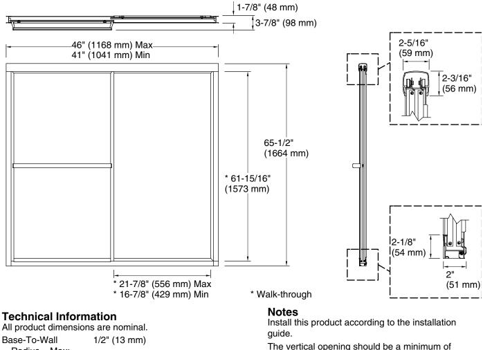
Radius – Max: Shower Ledge Min 1-7/8" (47 mm) Flat: Shower Wall Min 2-5/16" (59 mm) Flat: The vertical opening should be a minimum of 66-15/16" (1700 mm) to allow for installation clearance.
