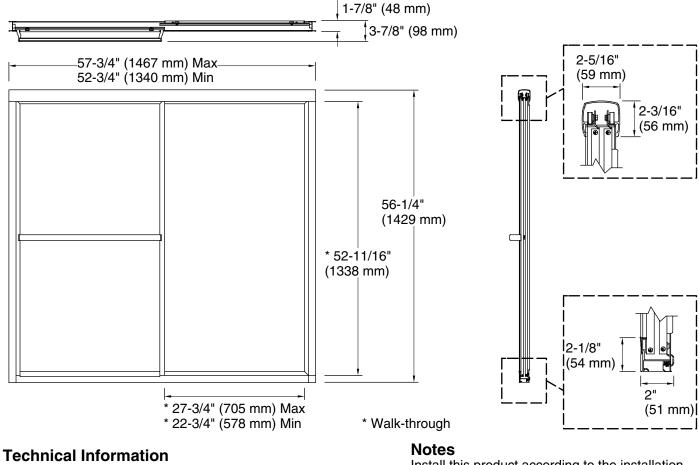
All product dimensions are nominal.Installation type:For bath installationOpening Width - Min:52-3/4" (1340 mm)Opening Width - Max:57-3/4" (1467 mm)Walk-through - Min:22-3/4" (578 mm)Walk-through - Max:27-3/4" (705 mm)Base-To-Wall Radius1/2" (13 mm)- Max:1/8" (3 mm)
