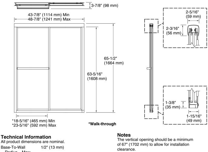
Base-To-Wall 1/2" (13 mm) Radius – Max: Shower Ledge Min 1-7/8" (48 mm) Flat: Shower Wall Min 2-5/16" (59 mm) Flat:
