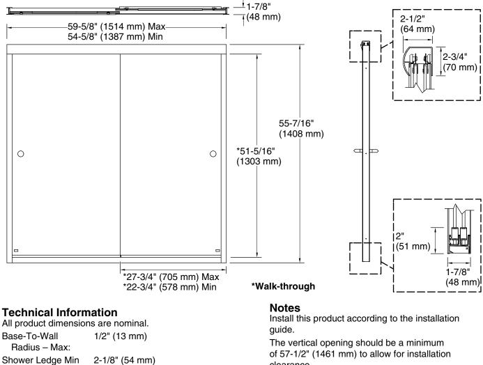
of 57-1/2" (1461 mm) to allow for installation clearance.
