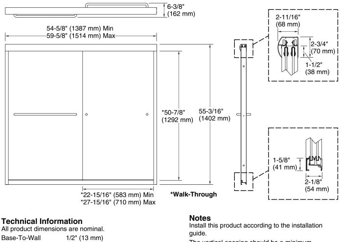
The vertical opening should be a minimum of 57-1/2" (1461 mm) to allow for installation clearance.
