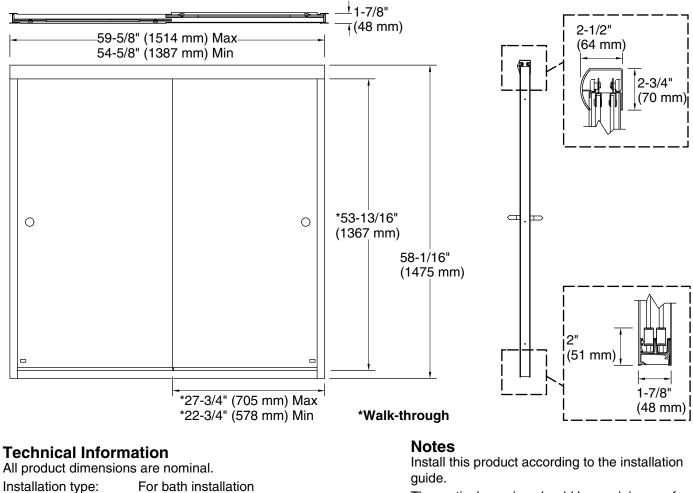
The vertical opening should be a minimum of 60-1/2" (1537 mm) to allow for installation clearance.
