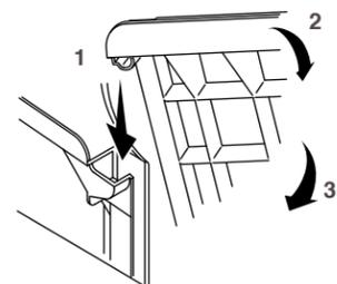
**16** The front edges should be flush, with no more than a 1/32" (1 mm) gap.
