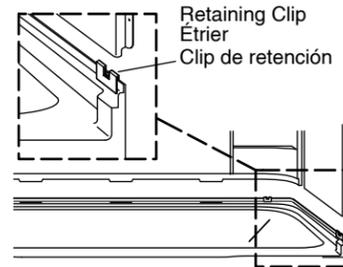
**13** Install the back wall. Insert the back wall tabs into the slots.
