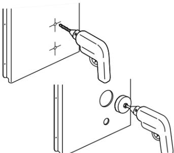
**15** Install the end walls. Engage the interlocks, pivot and snap the end walls into the retaining clips.
