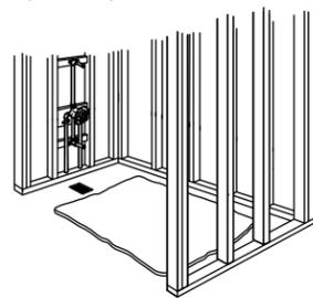
**6** Attach the apron brace, if provided. Lift and position the bath in the stud pocket.
