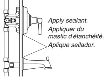
**22** After painting, apply 100% silicone sealant where the unit contacts the finished wall.
