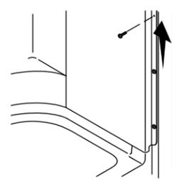
**18** Secure the walls to the studs along the top. Use shims as needed.
