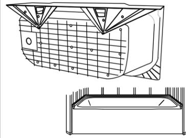
**7** Attach metal support clips to the flange at the locations shown in the roughing-in information.
