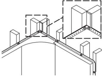
**20** Cover the framing with water-resistant wallboard. Install the finished wall material.
