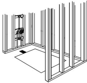
**5** Without a pad, we recommend the basin area be set in 1" (25 mm) to 2" (51 mm) of mortar cement.
