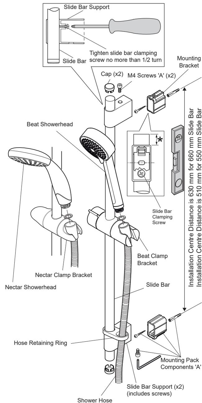
\* **Note!** Ensure an equal length of slide bar top and bottom.
