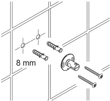
Drill the holes for the wall fixing bracket. Insert the wall plugs and fix the bracket to the wall using the screws supplied.
