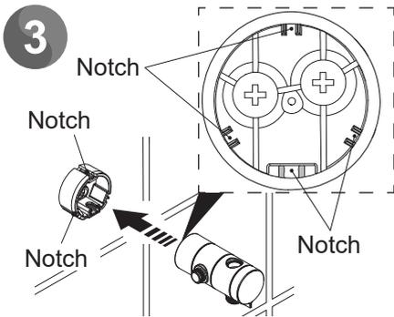
Slide the diverter partially over the wall plate ensuring the notches in the diverter lines up with the notches on the wall plate and fix temporarily in place.
