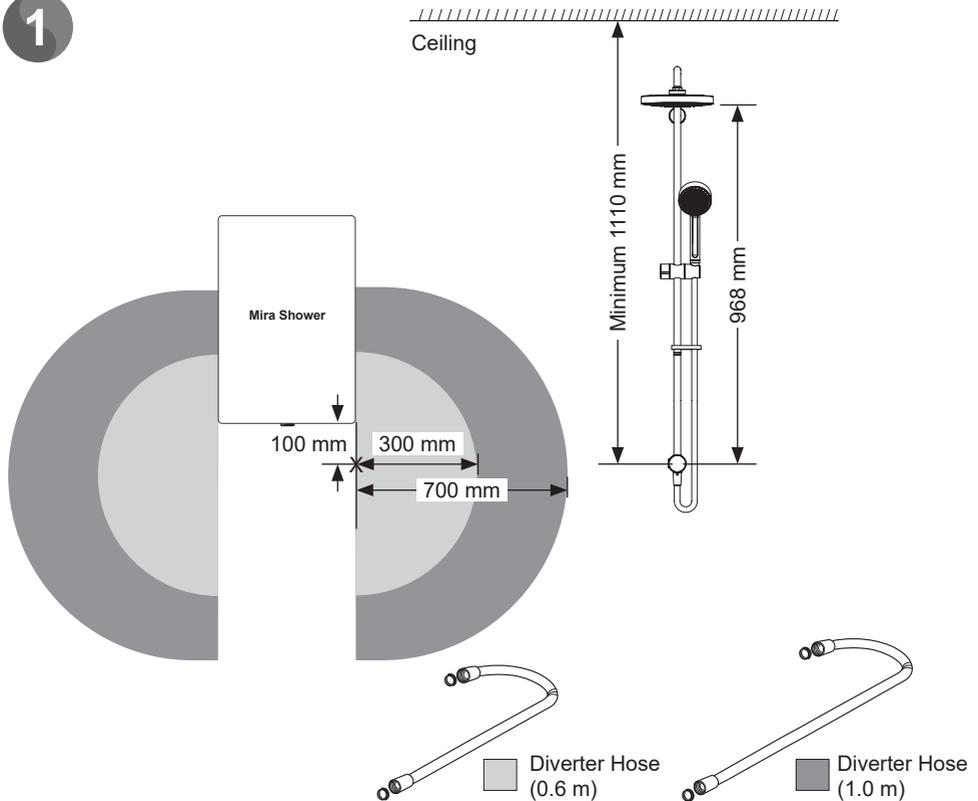
If the diverter is positioned outside of the light grey area as shown in the diagram a longer link hose is available up to 1.0 m max in length.
