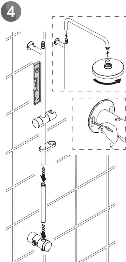
Fit the clamp bracket and hose retaining ring onto the middle bar, then screw into the lower bar. Loosely fit the wall bracket into the middle bar arm with the grubscrew hole at the top.
