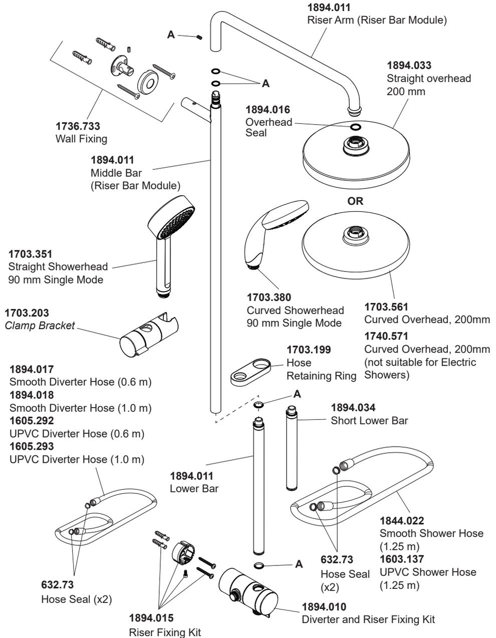
**1894.019** Seal and Grub Screw Pack (Components marked as 'A')
