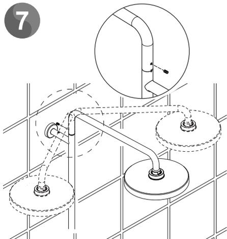
The overhead assembly can rotate 45° in either direction from centre.
