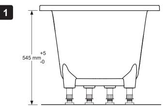
Make sure that the height of the bath has been set to the dimensions on the above diagram.
