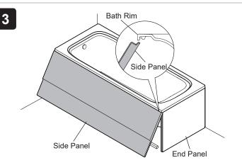
Slide the side panel under the rim of the bath. **Note:** If fitting an end panel, make sure that it fits inside the bath side panel.
