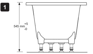
Make sure that the height of the bath has been set to the dimensions on the above diagram.
