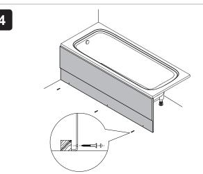
Secure the side panel to the floor baton through pre-drilled holes (to be determined by the installer) using the mirror screws (supplied).
