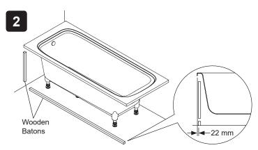
If necessary, for additional support, screw soft wooden batons to the floor and adjoining wall.
