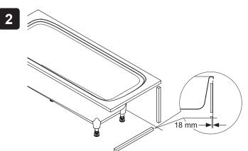
If necessary, for additional support, screw soft wooden batons to the floor and adjoining wall.
