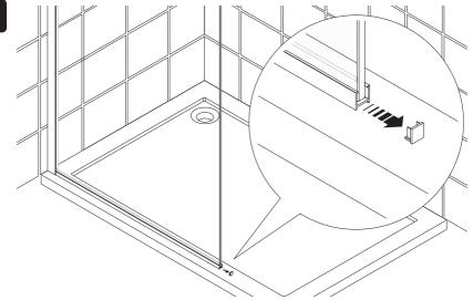
(a) If you are adding this panel to a pre-existing 8 mm frameless divider panel, you must remove the H section end cap.
