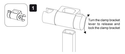
If required, install the clamp bracket on the end of the grab bar.
