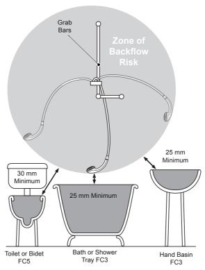
**Note!** There will be occasions when, for Fluid Category 3 installations, an outlet double checkvalve must be fitted, this will increase the required supply pressure typically by 10kPa (0.1 bar). Double check valves fitted in the inlet supply to the appliance cause a pressure build up, which affect the maximum static inlet pressure for the appliance and must not be fitted. For Fluid category 5 double check valves are not suitable.
