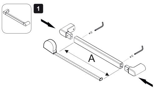
Measure the tube length 'A' and assemble the ends.
