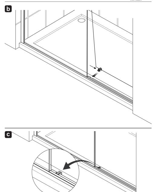
(a) Slide the glass guide assembly along the bottom of the door and then push it into the locator on the track (between the two splash seals).
