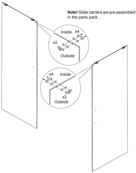
**Note!** To aid assembly, place the assembled door inside the enclosure prior to the fixed panel being installed.
