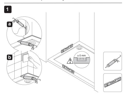
**Note!** Make sure that the walls have been tiled down to the tray. Make sure the tray is level. Make sure the walls are flat and square.
