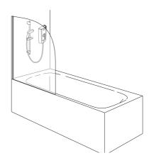
Decide on a suitable position for the shower unit and fittings leaving adequate space for maintenance. A suitable position for the shower will have a minimum clear distance of 100 mm around the shower unit to allow for cover removal and refitting. See *"Installation - Plumbing"* for further details.
